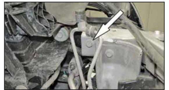
7. Remove the core support bolt shown.
