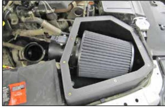
15. Install the K&N® mass air housing onto the mounting studs and into the K&N® air filter. Secure the housing to the studs with the provided hardware and then secure the air filter with the hose clamp provided.
