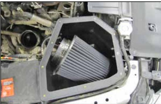
14. Set the K&N® air filter into the K&N® air box as shown.
