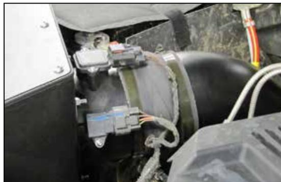
19. Reconnect the mass air sensor and temperature sensor electrical connection.
