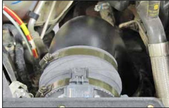
17. Install the K&N® intake tube into the factory turbo inlet hose and then connect the K&N® hose to the K&N® mass air sensor housing. Secure the intake tube with the hose clamps provided.
