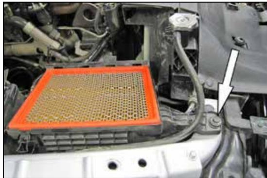
5. Remove the bolt which secures the lower air box to the core support.
