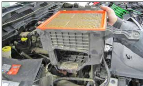
6. Lift up the lower air box to dislodge it from the mounting grommets and then remove it from the vehicle.
