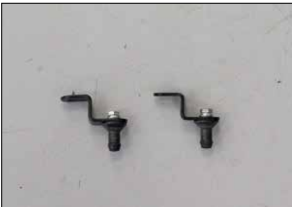
11. Install the two provided mounting studs onto the two heat shield brackets (070061) as shown.
