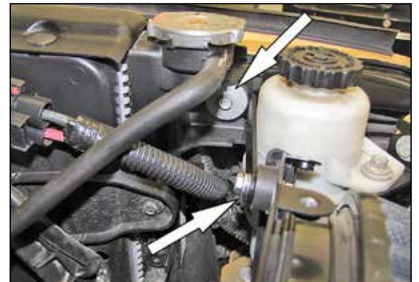
19. Install the heat shield bracket assembly onto the heat shield and radiator mount as shown. Secure the bracket with the factory bolt from step number 9 and the hardware provided.
