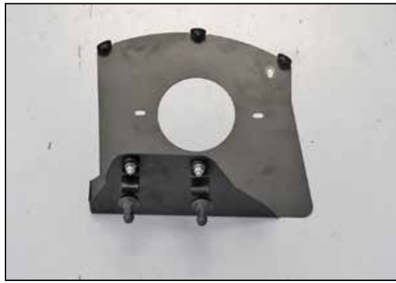
12. Install the two heat shield bracket assemblies onto the heat shield as shown.
