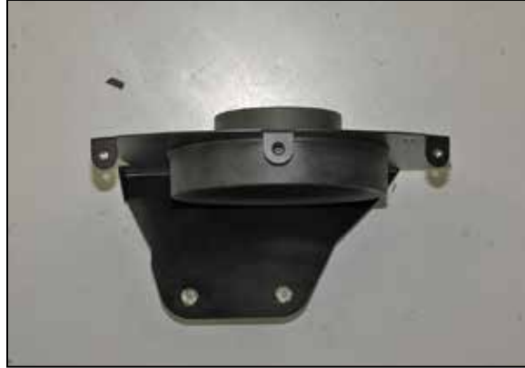
13. Install the provided filter adapter onto the heat shield as shown.
