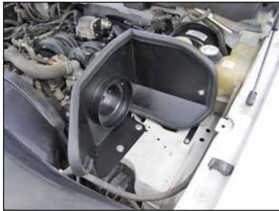
15. Set the heat shield onto the air box mounting plate so the inserts go into the mounting grommet holes. Secure the heat shield with the insert bolts and with the bracket to the inner fender with the provided hardware.
