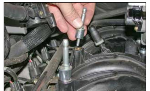
8. On vehicles with the heater hose and wiring harness attached to the air box studs, place a spacer under the two right side air box studs and reinstall the studs into the original location.
