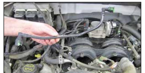
9. Release the crank case vent hose from the valve cover port and then remove the crank case hose from the vehicle.
