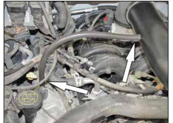
22. Install the provided crank case vent hose onto the vent port on the K&N® intake tube and then onto the vent on the valve cover.
