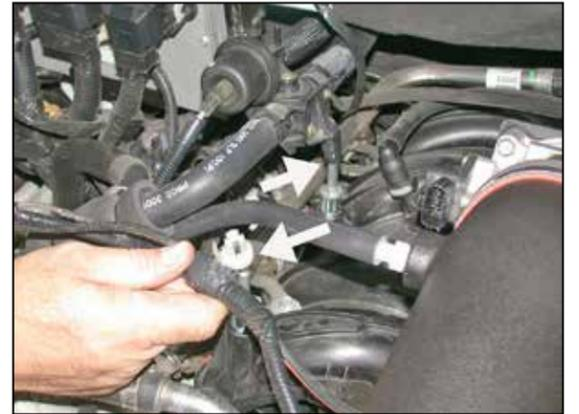
21. Reattach the heater hose and wiring harness to the studs installed in the previous step.
