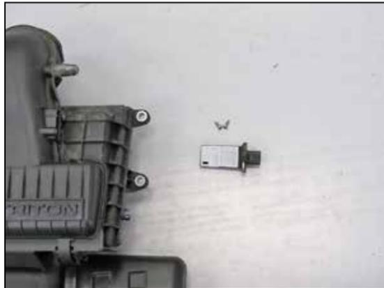
18. Remove the two screws securing the mass air sensor into the stock air filter housing and then remove the sensor from the vehicle.
