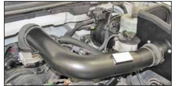
20. Install the K&N® intake tube into the 90° elbow hose and then into the hump hose, align for best fit and then secure with the provided hose clamp.
