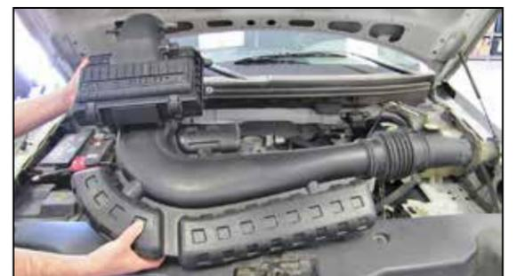
7. Remove the complete air box and intake snorkel assembly as shown.
