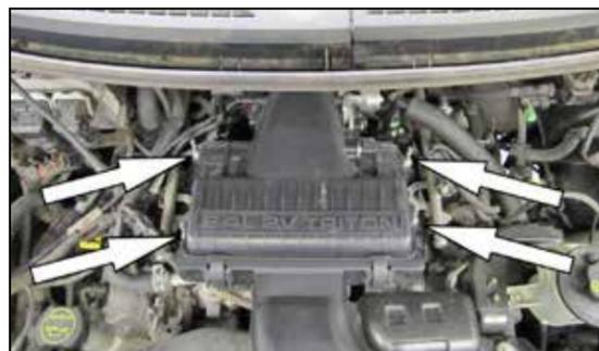
6. Remove the four bolts securing the air filter housing to the intake manifold.
