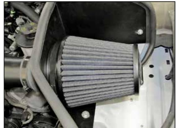
23. Install the K&N® air filter onto the filter adapter and secure with the provided hose clamp.
