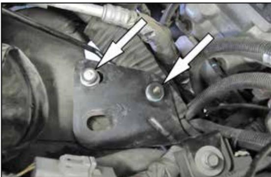
10. Install the two provided rubber mounted studs onto the air box mounting tray as shown.
