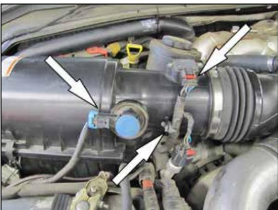
2. Disconnect the mass air sensor and filter minder electrical connections and unhook the wiring harness clip from the air box.
