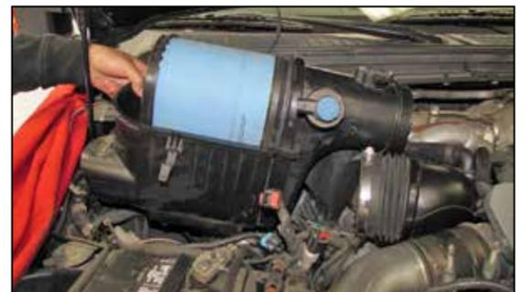
6. Lift up the lower air box to unhook it from the mounting grommets and then remove from the vehicle.
