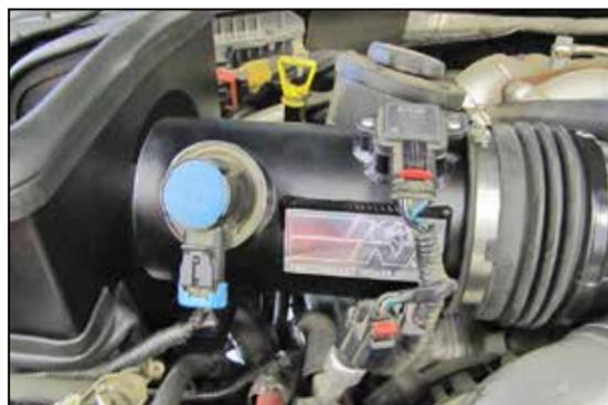
17. Connect the filter minder and mass air sensor electrical connections.
