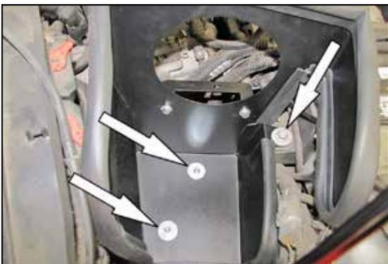
12. Install the heat shield assembly into position so that it rests onto the rubber mounted studs. Secure the heat shield onto the rubber mounted studs with the provided hardware and to the battery tray with the bolt removed in the previous step.
