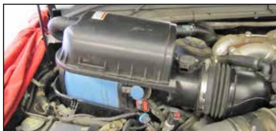
5. Release the two upper air box retaining clips and then remove the upper air box housing assembly as shown.
