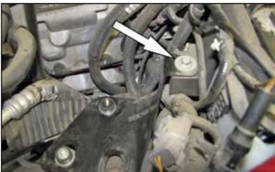
11. Remove the battery tray mounting bolt shown. **NOTE: This bolt will be reused.**
