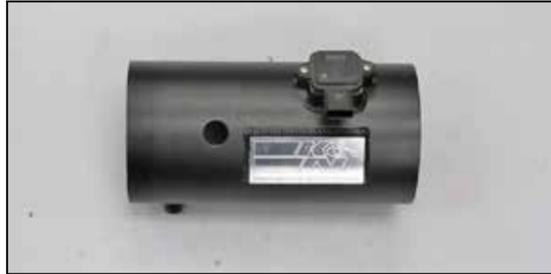
14. Install the mass air sensor into the K&N intake tube and secure with the provided screws.
