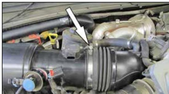
3. Loosen the hose clamp securing the inlet hose to the air box.
