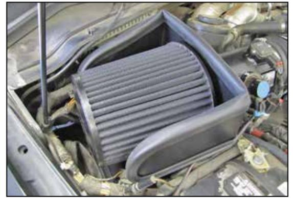
18. Install the K&N air filter and secure with the provided hose clamp.
