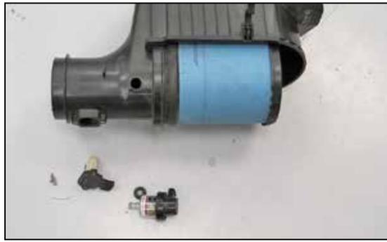
13. Remove the mass air sensor and filter minder along with the grommet from the factory air box as shown.
