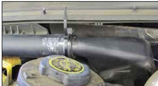
4. Unhook the warm air inlet tube from the firewall as shown.
