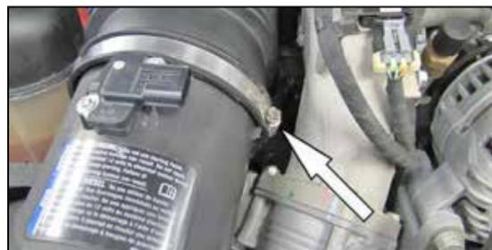
3. Loosen the hose clamp securing the factory intake tube to the air box.
