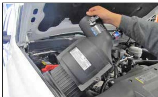
5. Lift up and remove the air filter assembly from the vehicle.
