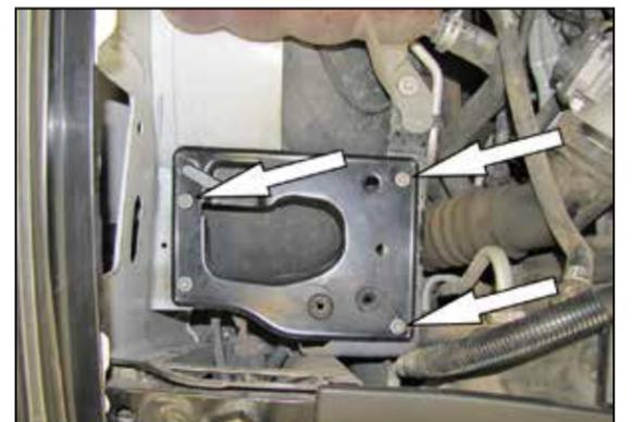
6. Remove the three bolts shown securing the air filter mounting plate.
