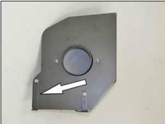
9. Install the provided heat shield bracket (070952) onto the heat shield and secure with the provided hardware.
