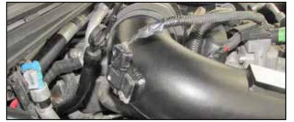
18. Connect the mass air sensor electrical connection.
