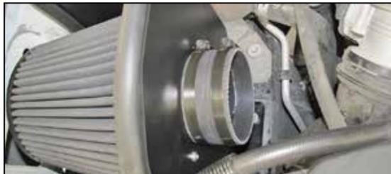
16. Install the provided coupling hose (08761) onto the filter adapter and secure with the provided hose clamp.
