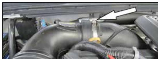
4. Loosen the hose clamp securing the intake tube to the turbo inlet and then remove the intake tube from the vehicle.
