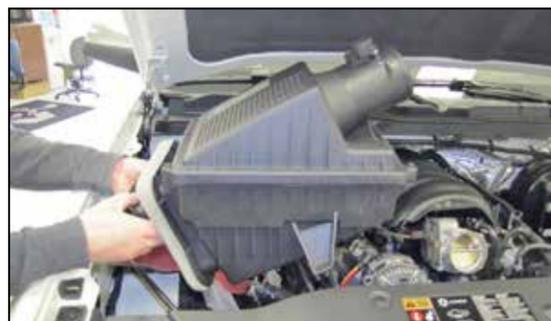
6. Pull up the air box to release it from the mounting grommets and then remove the factory air box from the vehicle.
