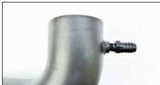
17. Apply thread sealant to the remaining CCV fitting and install it into the K&N intake tube.
