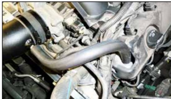
19. Install the provided CCV hoses onto the valve cover ports and connect the driver side hose to the K&N intake tube.
