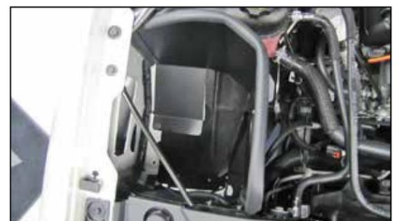
9. Install the heat shield assembly and secure to the air box mounting plate location using the three factory bolts from step #7.
