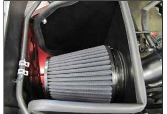
21. Install the K&N® air filter onto the filter adapter and secure with the provided hose clamp.
