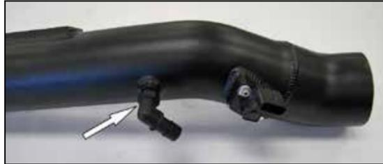
14. Install the 90° vent fitting into the K&N® intake tube as shown.
