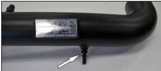
15. Install the quick connect fitting into the K&N® intake tube as shown.
