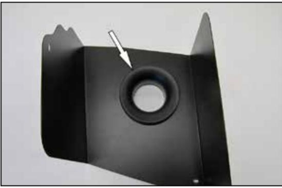
7. Install the filter adapter into the K&N® heat shield and secure with the provided hardware.
