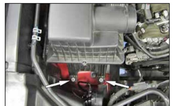
6. Remove the two nuts securing the air filter housing to the inner fender and then remove the housing from the vehicle.
