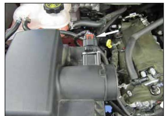
5. Release the red locking tab and then disconnect the mass air sensor electrical connection and unhook the harness from the air filter housing.
