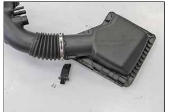
20. Remove the two screws securing the mass air sensor into the upper air box and then remove the mass air sensor from the air box.
