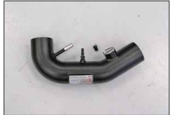
19. On vehicles equipped with an EVAP vent line, install the provided quick disconnect fitting into the K&N® intake tube. On vehicles not equipped with the EVAP vent line, install the provided 1/4npt plug into the K&N® intake tube.
