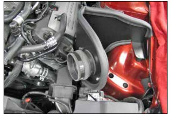
17. Install the provided silicone hump hose (08699) onto the filter adapter and secure with the provided hose clamp.
