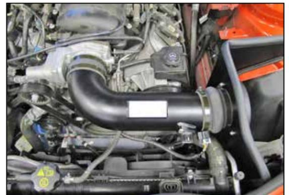
21. Install the K&N® intake tube assembly into the silicone hose at the filter adapter and then into the silicone hose at the throttle body and secure with the provided hose clamps.
