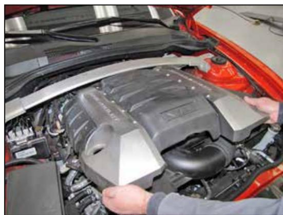
3. Remove the oil filler cap and then lift up and remove the engine cover. Reinstall the oil filler cap.
