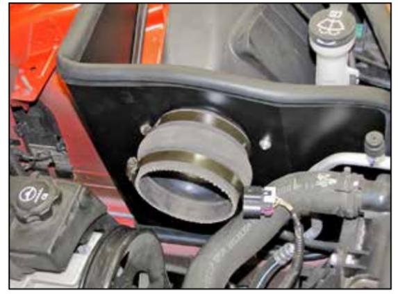
17. Install the silicone hose (08418) onto the filter adapter and secure with the provided hose clamp.
