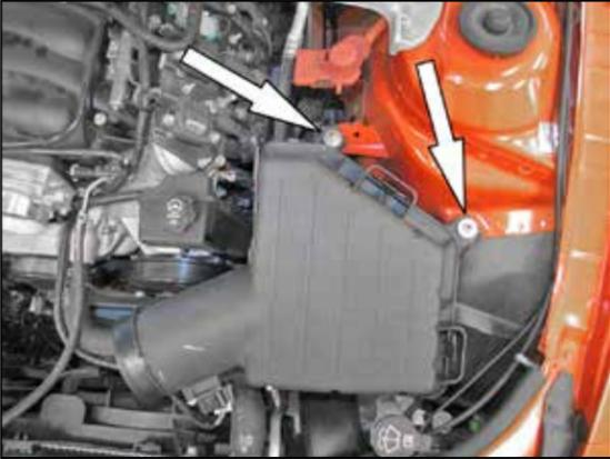
8. Remove the two air box retaining nuts shown.
