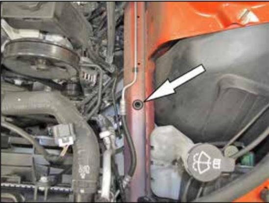
10. Remove the air box mounting grommet shown from the frame rail.
