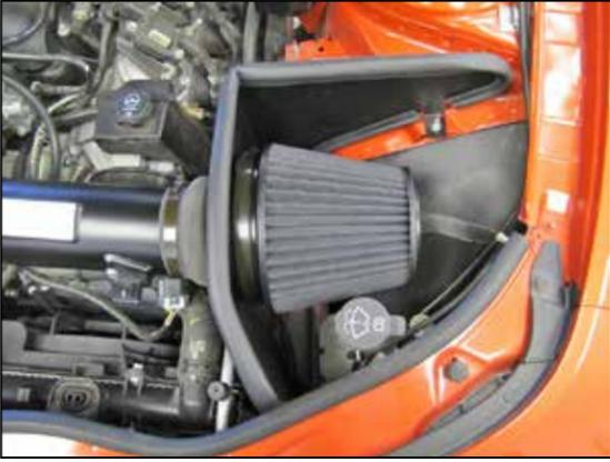
23. Install the K&N® air filter onto the filter adapter and secure with the provided hose clamp.
