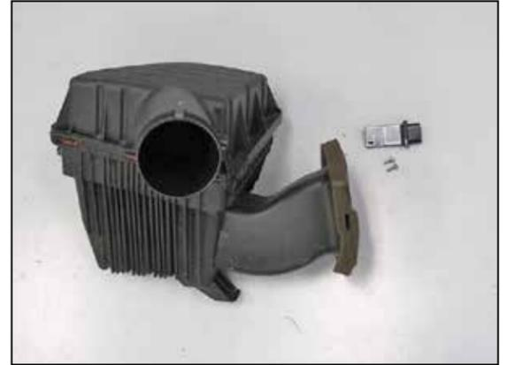
18. Remove the two screws and then remove the mass air sensor from the factory air box.
