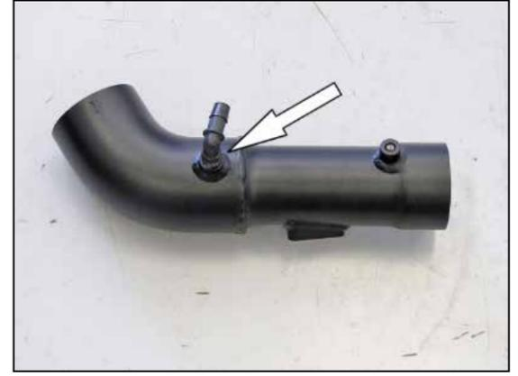
19. Install the provided 90° NPT vent fitting into the driver's side K&N® intake tube (27466) as shown.
