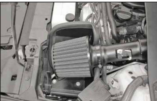
26. Install the K&N® air filter onto the K&N® intake tube and secure with the provided hose clamp.
