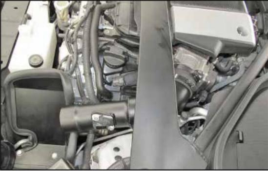
23. Install the K&N® intake tube into the silicone hose at the throttle body and align the bracket with the mounting hole in the heat shield. Adjust the tube and heat shield for proper fit and then secure with the provided hardware and hose clamp.
