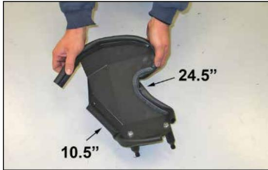
31. Install the provided edge trim onto the heat shield as shown.
