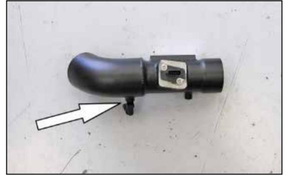
33. Install the provided 90° NPT vent fitting into the K&N® intake tube (27642) as shown.
