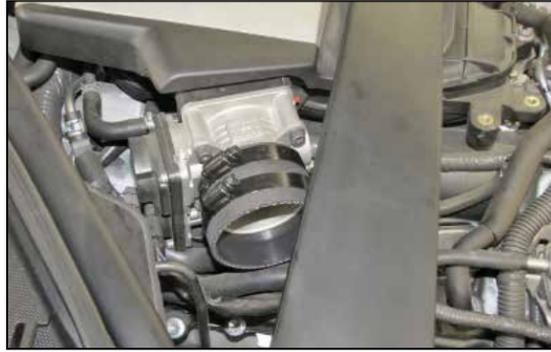
28. Install the coupling hose (084036) onto the passenger side throttle body and secure with the provided hose clamp.
