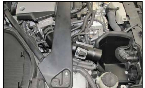
37. Install the K&N® intake tube into the coupling hose at the throttle body and align the bracket with the mounting hole in the heat shield. Adjust the tube and heat shield for proper fit and then secure with the provided hardware and hose clamp.
