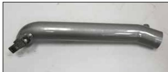
21. Remove the pressure sensor from the factory charge tube and then install it into the K&N charge tube using the provided hardware.
