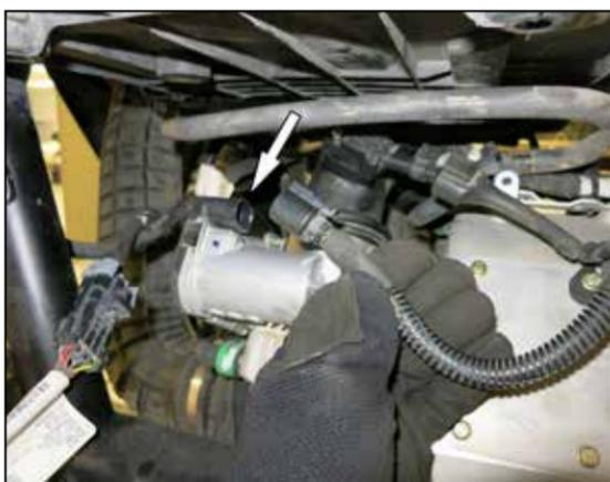
9. Disconnect the throttle body electrical connection
