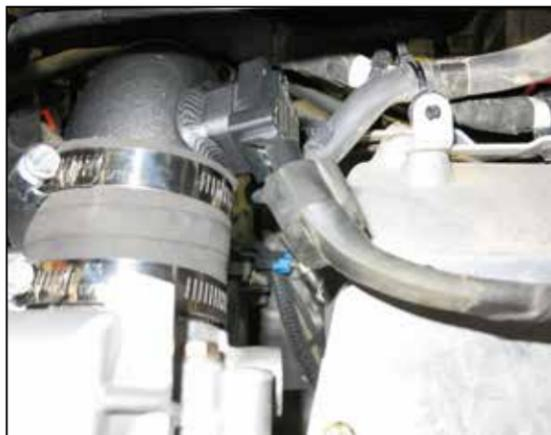
26. Reconnect the pressure sensor electrical connection.
