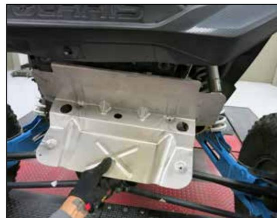
6. Remove the bolts that secure the muffler heat shield to the chassis and then remove the heat shield and set aside.
