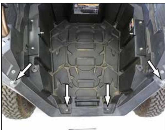
11. Reinstall the cargo box and secure with the factory hardware.
