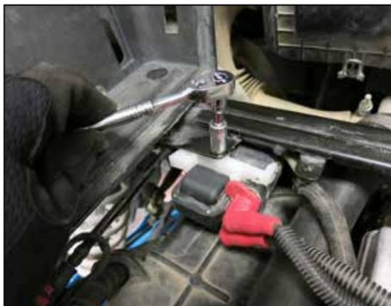
11. Remove the two bolts that secure the ignition coil to the chassis.
