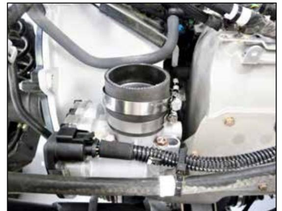
6. Install the straight coupler onto the throttle body and secure with the provided hose clamp.
