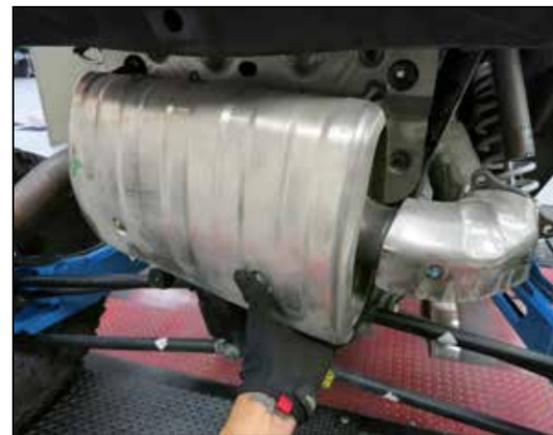
5. Remove the three nuts that secure the muffler to the exhaust pipe. Remove the mounting spring on the left side of the muffler and then remove the complete muffler assembly from the vehicle.
