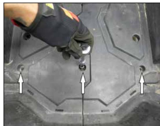
7. Remove the three bolts shown that secure the cargo bed to the support bracket.
