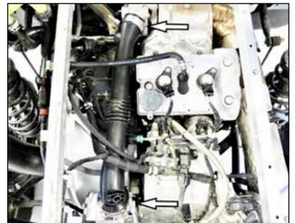
5. Loosen the two hose clamps that secure the charge tube to the turbo outlet and intake inlet, then remove the charge tube from the vehicle.
