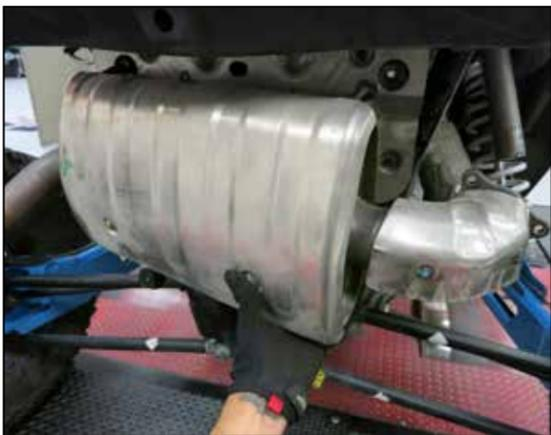
32. Reinstall the muffler using all of the factory hardware and springs.
