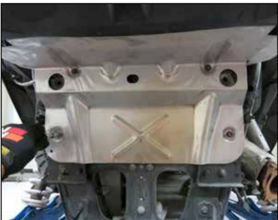
31. Reinstall the muffler heat shield using the factory bolts.
