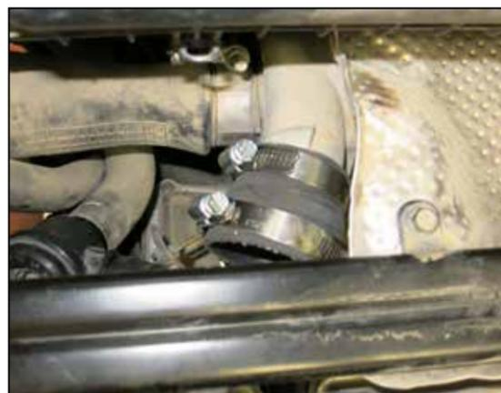
20. Install the step coupler onto the turbo outlet and secure with the provided hose clamp.
