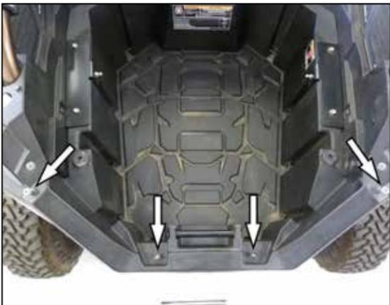
2. Remove the four bolts that secure the cargo box and then remove the cargo box from the vehicle.
