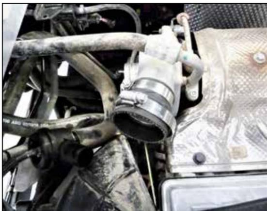
7. Install the step coupler onto the turbo outlet and secure with the provided hose clamp.
