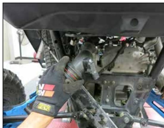
19. Carefully guide the factory charge tube towards the rear of the vehicle past the throttle body and out.
