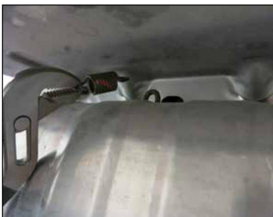
4. Remove the spring that secures the top of the muffler to the chassis.
