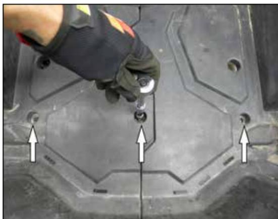
30. Reinstall the three-cargo box mounting bolts.
