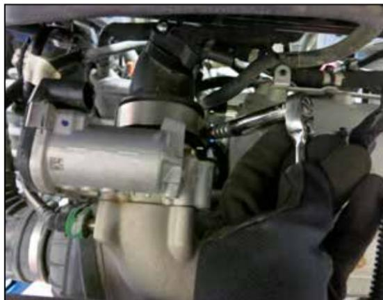
15. Loosen the hose clamp that secures the factory charge pipe to the throttle body.
