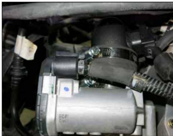
27. Reconnect the throttle body electrical connection.
