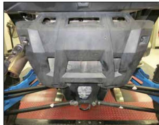
33. Reinstall the exhaust system cover over the muffler with the factory bolts.
