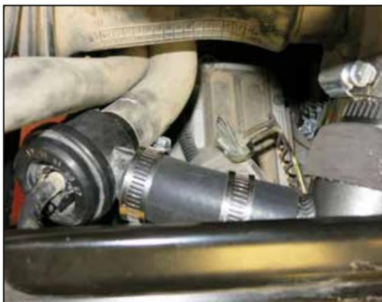
25. Using the provided BOV hose and clamps, secure the BOV to the K&N charge pipe.
