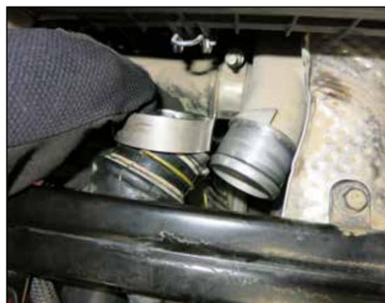
18. Separate the charge tube from the turbo and remove the clamp.
