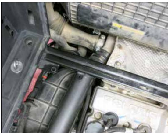
23. Guide the K&N charge tube from the rear off the vehicle into position into the coupler at the turbo.
