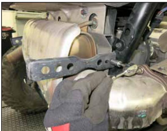
3. Remove the bolt that secures the muffler cover bracket to the chassis.
