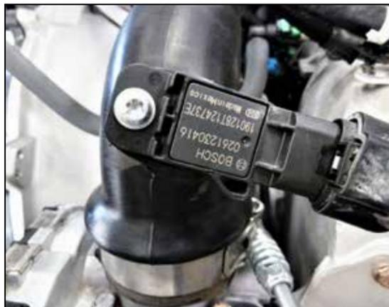
4. Remove the screw that secures the charge pipe pressure sensor, Remove the sensor from the charge tube and set on top of the engine to the side.
