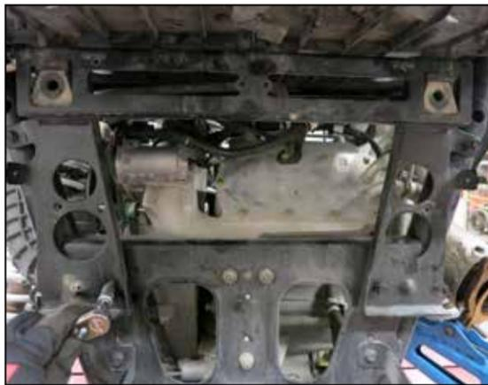
29. Reinstall the cargo box/exhaust support bracket to the chassis and secure with the factory bolts.
