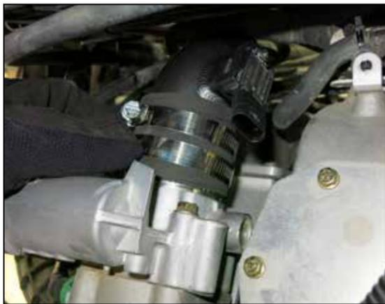
24. Position the tube onto the throttle body and slide the coupler over the throttle body into position. Adjust the tube for best position and then tighten all the remaining hose clamps.
