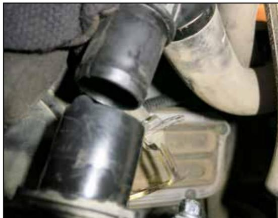
17. Loosen the clamp that secures the BOV and then separate the BOV from the factory charge tube.
