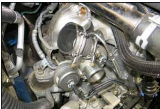
11. Install the provided step coupler into the turbo outlet with the provided clamps, do not tighten the clamps.
