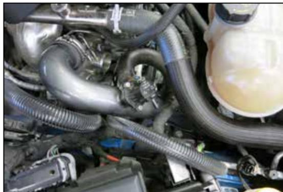
13. Install the K&N hot side charge tube into the couplers, align the tube for best fit and then tighten all the hose clamps. Reconnect the BOV electrical connection.
