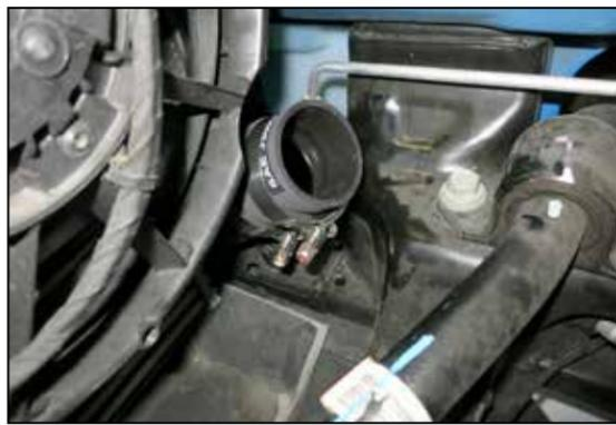
12. Install the provided hump coupler onto the hot side of the intercooler with the provided clamps, do not tighten the clamps.
