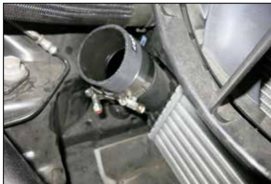
15. Install the provided step coupler onto the cold side of the inter cooler with the provide clamps, do not tighten.
