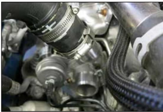
7. Loosen the hose clamps that secure the hot side charge tube to the turbo and intercooler and then remove the charge tube from the vehicle.
