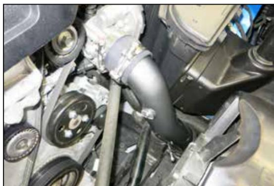
16. Install the K&N cold side charge tube into the couplers, align for best fit and then tighten the clamps.
