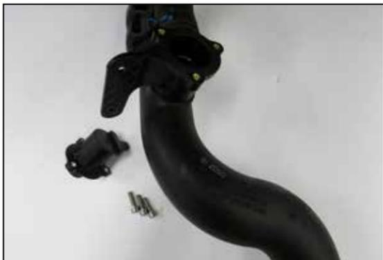
8. Remove the three bolts that secure the BOV to the factory charge tube and remove the valve from the tube. Release the spring clamp and disconnect the BOV hose from factory hot side charge tube
