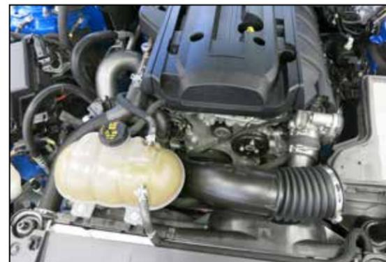
18. Reinstall the complete intake system and reconnect the factory BOV hose to the intake tube.
