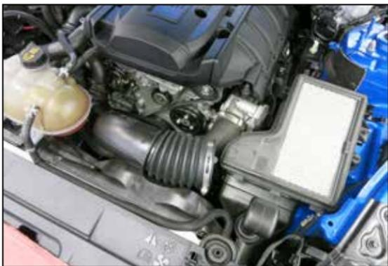
2. Loosen the hose clamp that secures the intake tube to the upper air filter housing and then release the clips that secure the upper housing to the lower housing.
