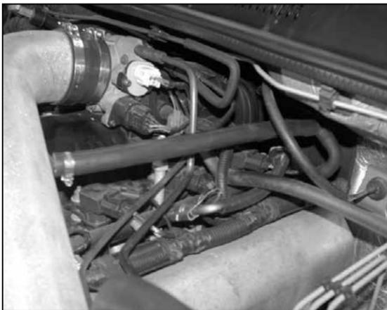
23. Connect the other end of the silicone hose to the vent on the K&N® intake tube as shown.
