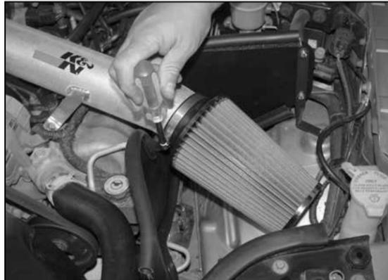
27. Install the K&N® air filter on the K&N® intake tube and secure with the provided hose clamp as shown.
