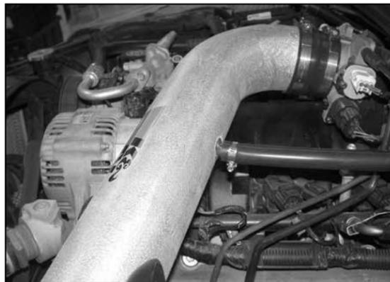
26. On 2003 models connect the crank case vent hose to the K&N® intake as shown.
