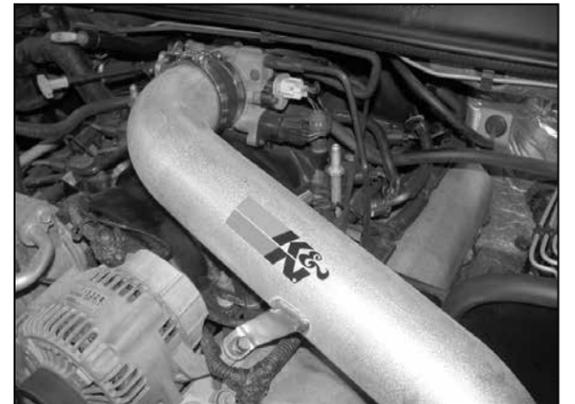
20. Slide the K&N® intake tube into the silicone hose on the throttle body and secure the bracket to the alternator using the stock bolt removed in step 18.
