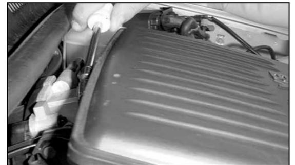
6. Loosen the hose clamp on the intake tube at the throttle body.
