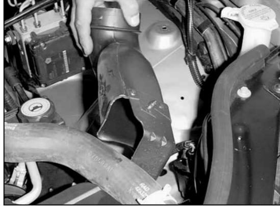
12. Release the clip that retains the air inlet duct to the radiator core support and remove the air inlet duct.
