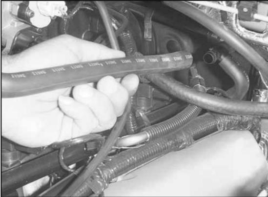
9. Detach the OE crankcase vent hose from the "T" fitting.
