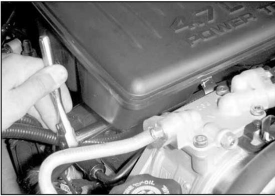
7. Loosen and remove the 2 bolts that retain the intake tube to the intake manifold.
