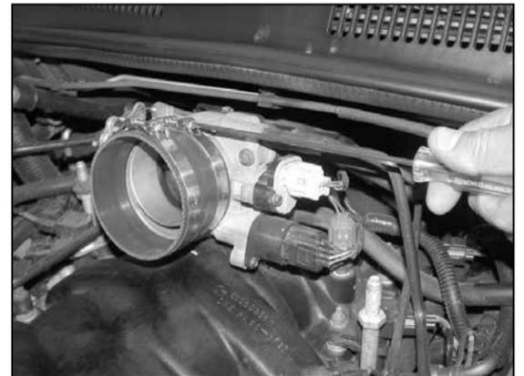
19. Install the provided silicone step hose and hose clamps onto the throttle body as shown.
