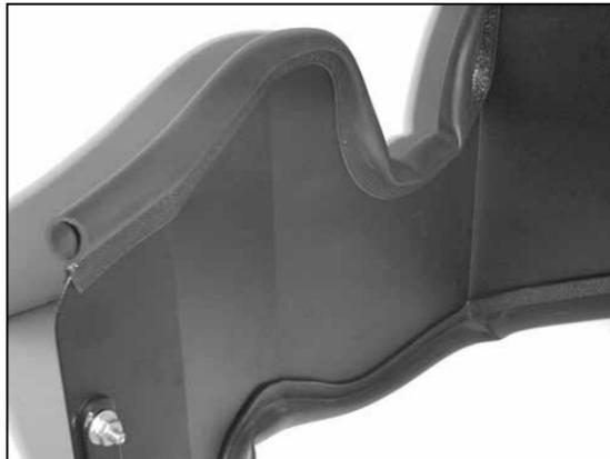
14. Install the trim seal onto the heat shield as shown.
