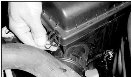
4. Release the 4 over center clips that retain the airbox top to airbox base.
