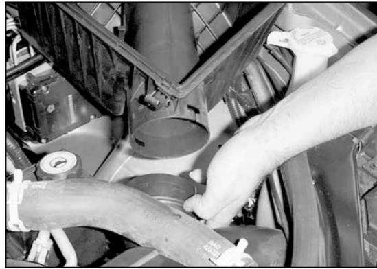
11. Detach the air inlet duct from the air box base and remove the air box base.
