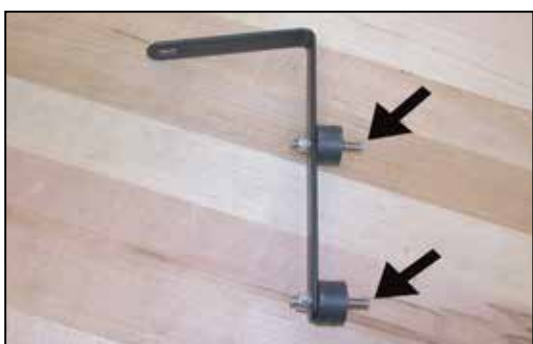
13. Install the rubber mounted studs onto the "L" bracket using the provided hardware but do not completely tighten at this time.
