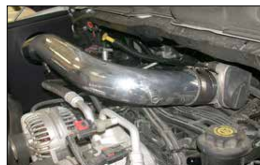
26. Slide the intake tube into the heat shield then slide the tube into the silicone hose on the throttle body as shown, but do not tighten completely at this time.
