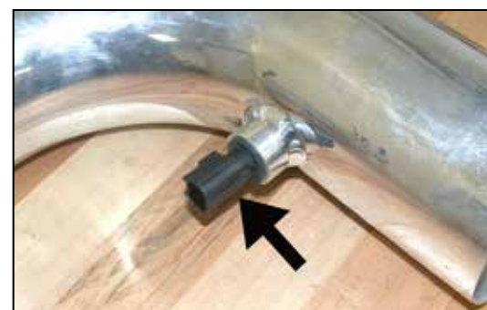
25. Slide the air temperature sensor into the silicone hose as shown. NOTE: The plastic cage on the end of the air temperature sensor is very fragile so take care when installing the air temperature sensor into the silicone hose.
