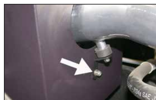
27. Secure the angle bracket to the heat shield using the provided hardware as shown, but do not tighten completely at this time.
