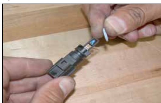
21. Remove the o-ring from the stock air temperature sensor as shown. NOTE: Be careful not to damage the o-ring.
