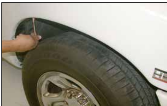
11. Reinstall the inner fender valance using 6 of the original 8 bolts removed in step 9.
