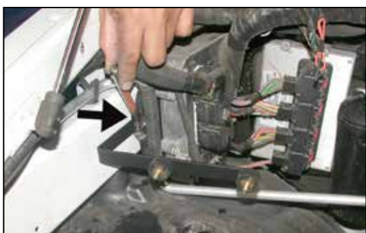
14. Secure the "L" bracket assembly to the threaded hole from step 12 using the original bolt as shown.
