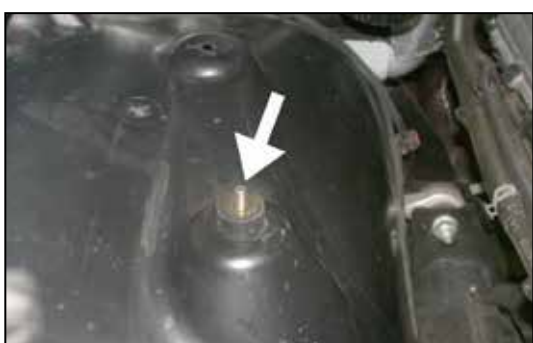
15. Secure the provided rubber mounted stud to the hole on the plastic inner fender valance using the provided hardware, but do not completely tighten at this time.
