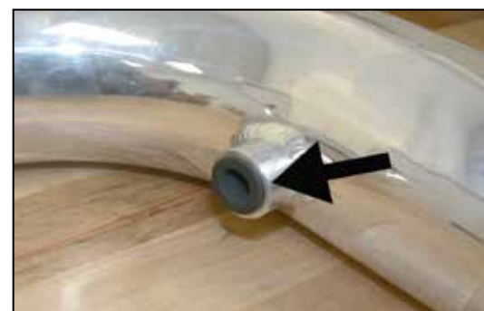
24. Install the provided silicone hose into the vent on the K&N® intake tube as shown.
