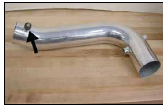
22. Install the rubber mounted stud into the threaded boss on the K&N® intake tube as shown.
