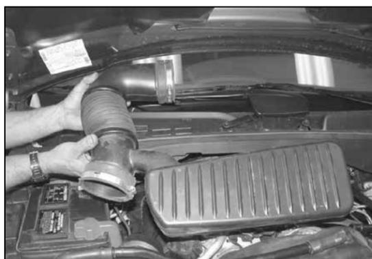
3. Loosen the intake tube hose clamps and remove the intake tube assembly from the vehicle.
