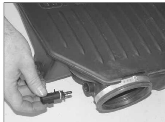
15. Twist the temp sensor counter clockwise to unlock and remove the temp sensor from the factory resonator.
