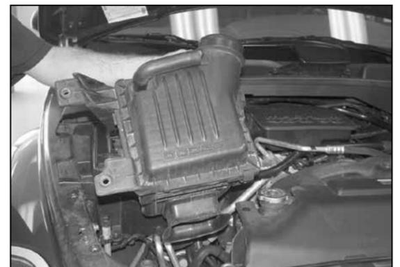
5. Pull up firmly to dislodge the airbox from mounting grommet, and remove the airbox from the vehicle.
