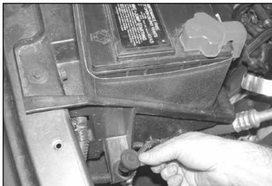
12. Install the 3/8" threaded insert provided into the airbox mounting grommet hole vacated in step #11.
