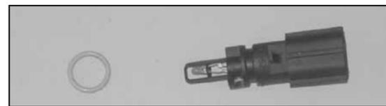
16. Remove the O-ring from the air temp sensor as shown.
