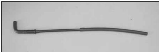
7c. Install the provided silicone hose onto the cut crankcase vent hose as shown and then reconnect the hose assembly onto the intake manifold.
