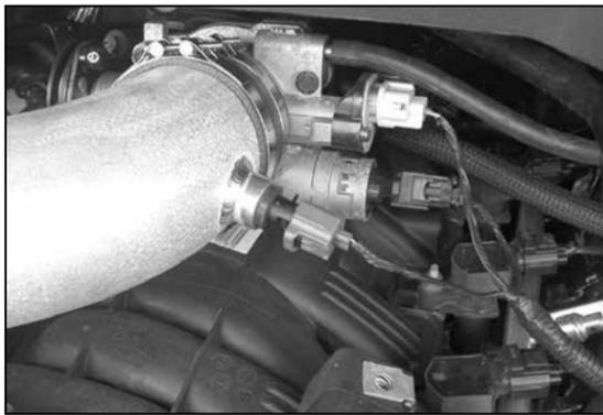
25. Reconnect the air temperature sensor electrical connection as shown.
