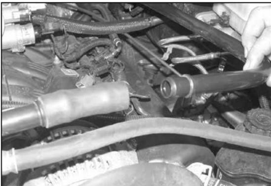
2. On 2005 and earlier vehicles, disconnect the crankcase vent tube from the vent hose junction above the alternator.
