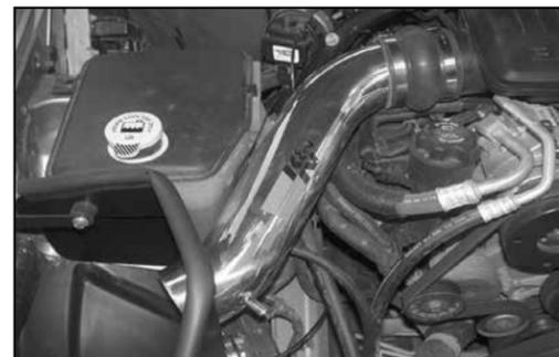
24. Install the K&N® intake tube into the silicone hose at the throttle body and onto the bracket. Secure the tube with the provided hose clamp and hardware.
