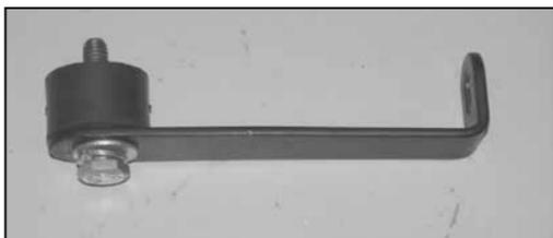
13. Install the 1/4"-20 male/female rubber mounted stud onto the "L" bracket (070952) with the provided hardware as shown.
