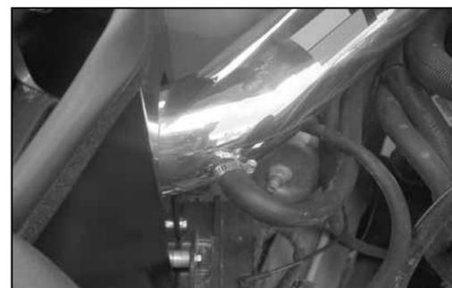
25. Connect the crankcase vent hose onto the K&N® intake tube as shown and secure with the provided hose clamp.
