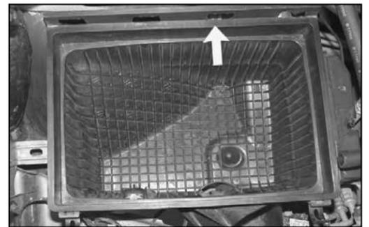
8. Remove the airbox mounting bolt shown.
