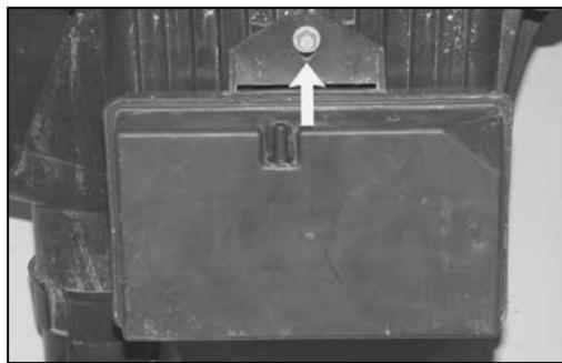
16. On vehicles equipped remove the bolt which secures the vacuum reservoir to the airbox and then remove the reservoir from the airbox.
