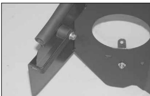
14. Install the bracket/rubber mounted stud assembly onto the heat shield as shown using the provided hardware.
