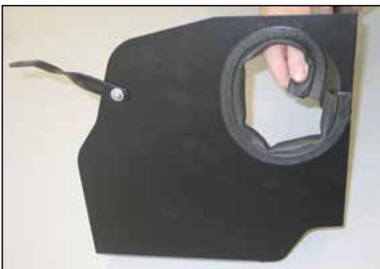
14. Install the provided edge trim into the hole of the heat shield as shown. NOTE: Some trimming of the edge trim will be necessary.
