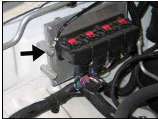
17. Remove the forward/upper ECU mounting bolt and ground strap.
