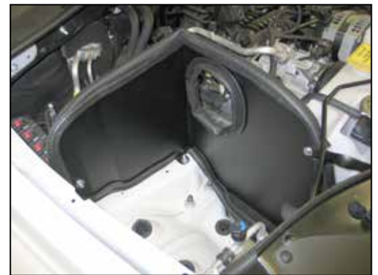
22. Install the heat shield assembly into the vehicle. Secure the rear of the heat shield to the mounting bracket installed onto the ECU. Secure the front heat shield mounting bracket to the radiator core support at the drilled location. Secure the bottom of the heat shield to the inner fender stud.
