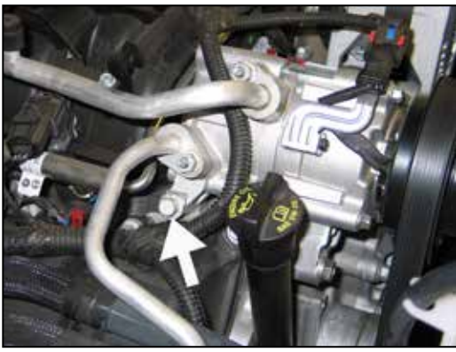
10. Remove the lower rear A/C compressor mounting bolt shown. NOTE: This bolt will be reused in the next step.
