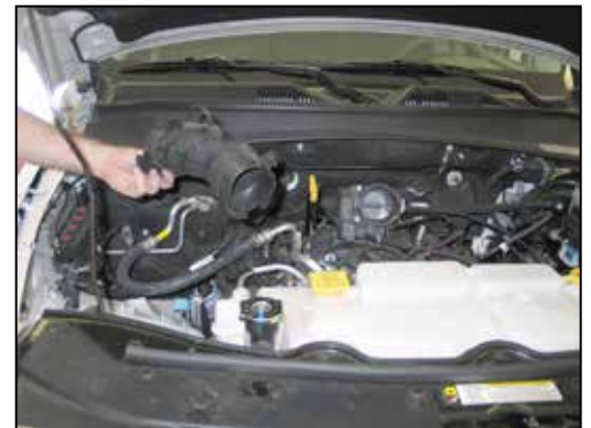
21. Remove the fresh air supply duct from the radiator core support as shown.
