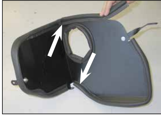
16. Install the provided edge trim onto the heat shield as shown. NOTE: Some trimming of the edge trim will be necessary.
