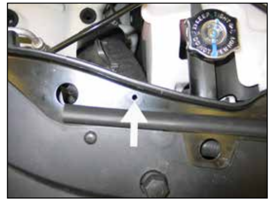
20. Drill a 1/4" id hole at the marked location.
