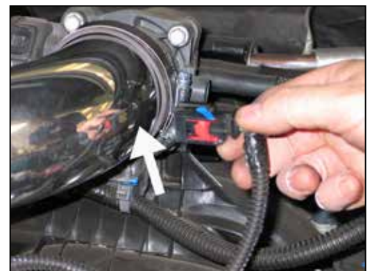
23. On vehicles equipped with an inlet air temperature sensor, install the K&N® intake tube into the silicone hose at the throttle body. Position the inlet air temperature sensor electrical connection for best fit. Mark the location for drilling.
