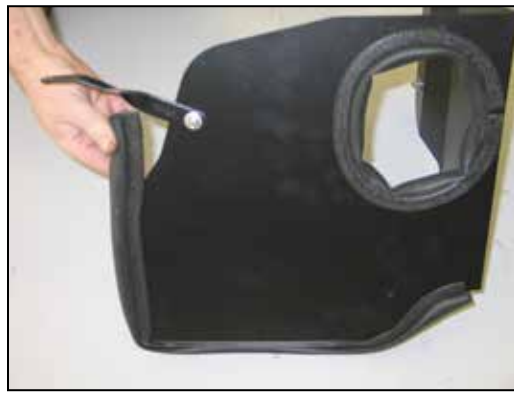
15. Install the provided edge trim onto the heat shield as shown. NOTE: Some trimming of the edge trim will be necessary.
