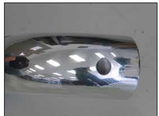
24. Remove the K&N® intake tube and drill a 3/4" id hole into the K&N® intake tube at the marked location. NOTE: Be sure to remove all burrs and shavings.
