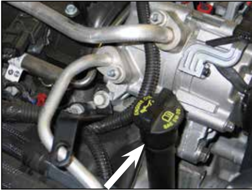
11. Install the tube mounting bracket (010064) onto the A/C compressor and secure with factory bolt removed in the previous step.
