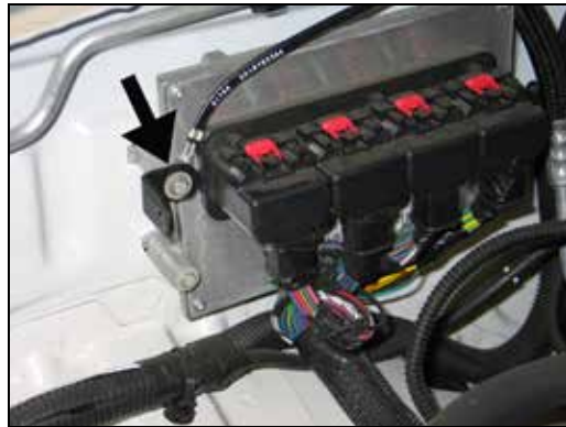
18. Install the heat shield mounting bracket (070066) onto the ECU and secure with the factory bolt removed in the previous step. NOTE: Be sure to place the slotted end of the bracket on to the ECU. Be sure to place the ground strap between the bracket and ECU as shown.
