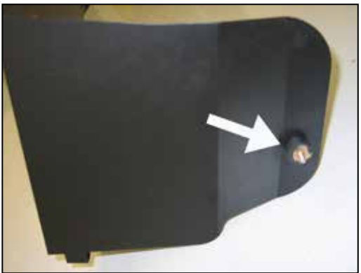
13. Secure the provided rubber mounted stud to the heat shield as shown using the provided hardware.
