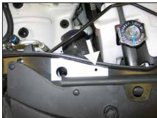
19. Using the provided template, place a mark onto the radiator core support for a hole to be drilled for the heat shield mounting bracket.
