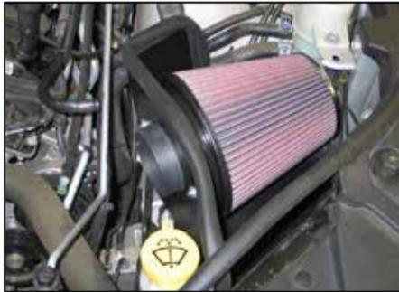
16. Set the heat shield/filter assembly into position so that the mounting grommets slide over the outer air box mounting studs.
