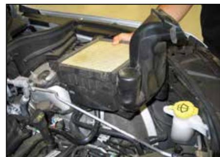
8. Lift up the lower air box to dislodge it from the mounting grommets, then remove the lower air box from the vehicle.
