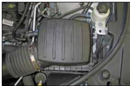
5. Release the two clips that secure the upper air box.
