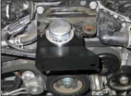
10. Install the provided tube mounting bracket (083150) onto the air injection pump mounting studs, reinstall the air injection pump and secure with the factory mounting nuts from step #9.
