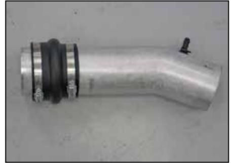
22. Slide the provided silicone hump hose (5-576) all the way onto the K&N® intake tube #27446 as shown.
