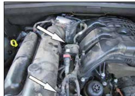
6a. If equipped with an EVAP solenoid attached to the intake tube, unhook the solenoid from the intake tube and secure it to the engine with the provided tie wrap.
