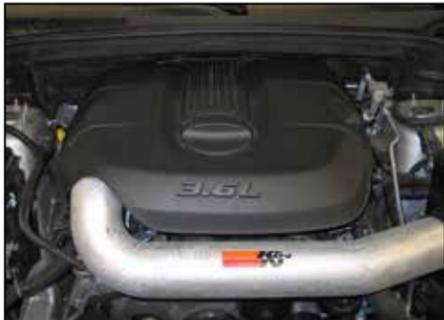
27. Adjust the intake kit for proper fit and then secure the mounting hardware and hose clamps. Reinstall the factory engine cover.
