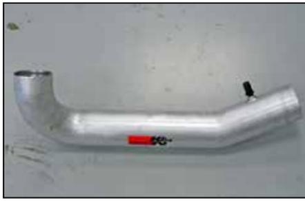
19. Install the provided ¼ npt vent fitting into the K&N® intake tube #27447 as shown.
