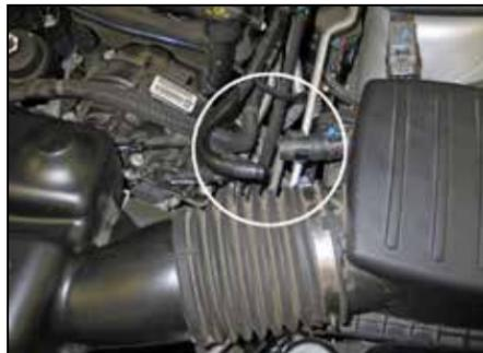
4. Disconnect the crank case vent tube from the air box as shown.
