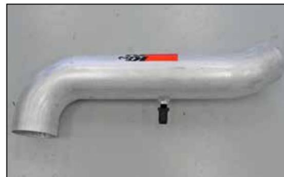
19. Install the provided NPT vent fitting into the K&N® intake tube as shown.
