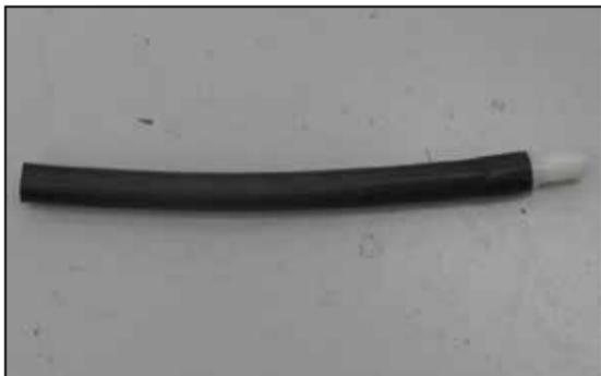
24. Install the provided hose mender into the provided crankcase vent hose as shown.
