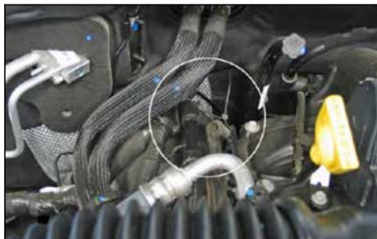
3. Disconnect the crankcase vent hose at the rear of engine, leaving elbow attached to cylinder head.
