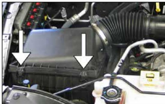
4. Release the two upper airbox retaining clips.
