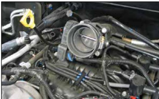
8. Install the silicone hose (084034) onto the throttle body and secure with the provided hose clamp.
