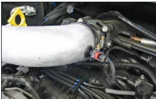
27. Reconnect the inlet air temperature sensor electrical connector as shown.
