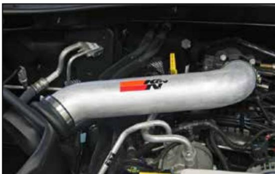
23. Install K&N® intake tube into the silicone hose at the filter adapter and then into the silicone hose on the throttle body. Secure the intake tube with the provided hose clamps.
