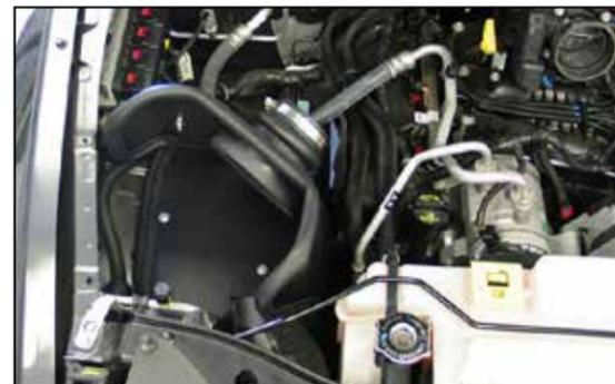
18. Place the heat shield assembly into vehicle so the mounting standoffs are secured in the factory airbox mounting grommets. Secure the mounting bracket to the ECU using the bolt removed in step #17.
