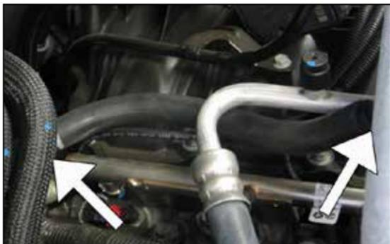
25. Install the crankcase vent hose onto the NPT fitting on the K&N® intake tube. Install the hose mender end into the factory elbow on the valve cover.
