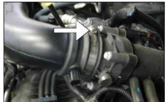
5. Loosen hose clamp at throttle body.
