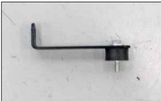
11. Install rubber mounted stud onto the heat shield mounting bracket (070952) as shown using the provided hardware.
