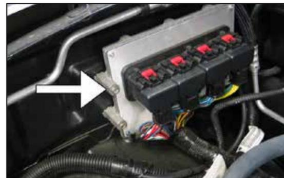
17. Remove the front upper ECU mounting bolt shown.
