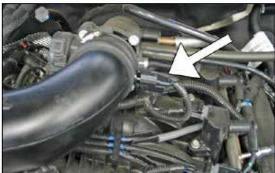
2. Release the red locking tab and then disconnect the inlet air temp sensor electrical connection.
