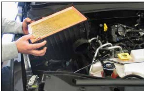
7. Lift up the lower airbox assembly to dislodge it from the mounting grommets, then disconnect the fresh air duct from the lower airbox and then remove the lower airbox from the vehicle.
