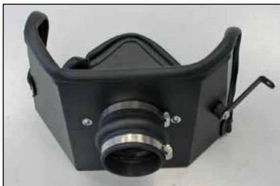
13. Install the silicone hump hose (5-576) onto the filter adapter and secure with provided hose clamp.
