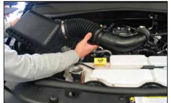
6. Remove the upper airbox and intake tube assembly from the vehicle.
