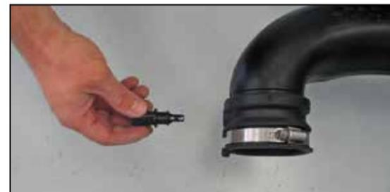
21. Remove inlet air temperature sensor from factory tube as shown.
