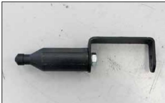
14. Install the heat shield mounting standoff onto the mounting bracket (083151) using the provided hardware as shown.
