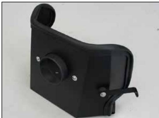
12. Install the heat shield mounting bracket assembly onto the heat shield using the provided hardware.
