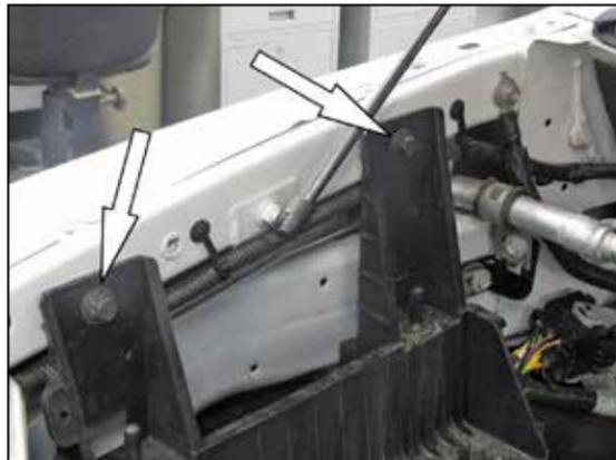
14. Remove the two factory air box mounting bracket bolts shown.
