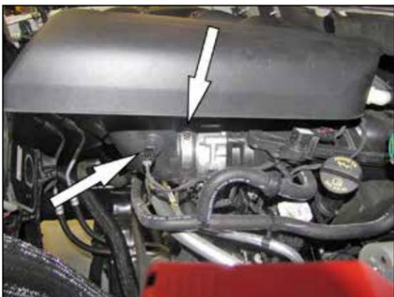
2. Disconnect the Inlet air temperature sensor electrical connection and loosen the hose clamp securing the intake plenum to the throttle body.
