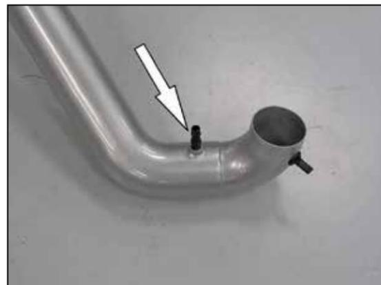
21. Install the provided vent fitting into the K&N® intake tube as shown.
