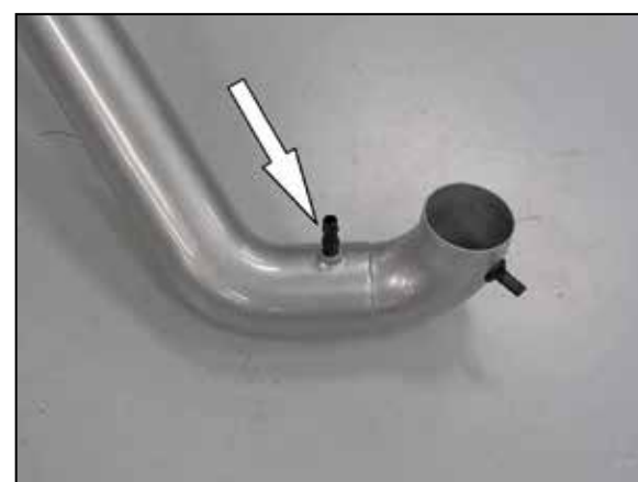
21. Install the provided vent fitting into the K&N® intake tube as shown. NOTE: Plastic NPT fittings are easy to cross thread. Install the vent fitting "hand" tight, then turn it two complete turns with a wrench.
