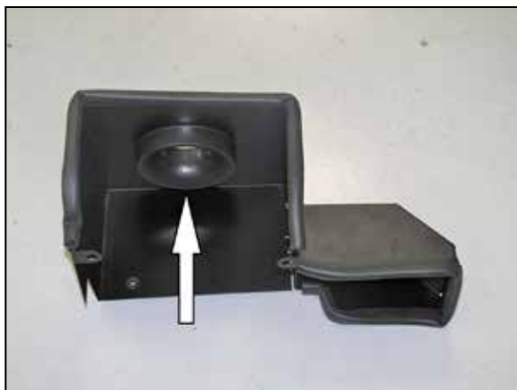
12. Install the K&N® air filter adapter into the heat shield and secure with the provided hardware.
