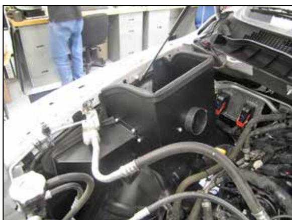
15. Set the heat shield into position on the factory air box mounting bracket and then secure with the factory bolts removed on step #14.
