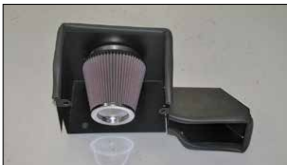
13. Install the K&N® air filter onto the filter adapter and secure with the provided hose clamp. NOTE: Drycharger® air filter wrap; part # RF-1042DK is available to purchase separately. To learn more about Drycharger® filter wraps or look up color availability please visit http://www.knfilters.com ®.
