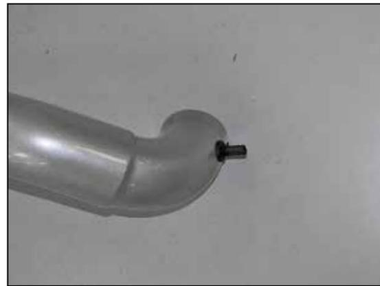
20. Install the inlet air temperature sensor into the grommet installed into the K&N® intake tube.
