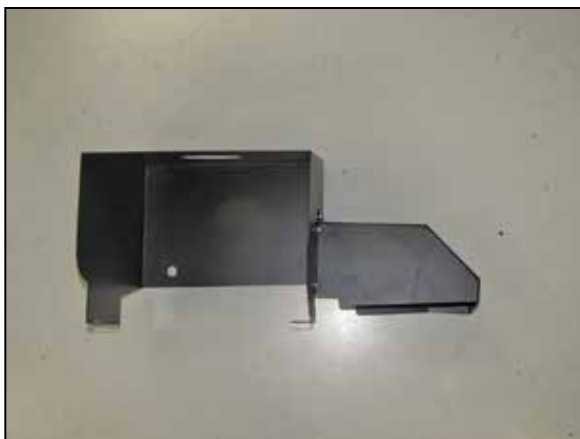
7. Install the K&N® fresh air intake scoop onto the K&N® heat shield and secure with the provided hardware.
