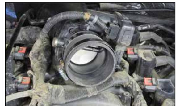
5. Install the provided coupling hose (08496) onto the throttle body and secure with the provided hose clamp.
