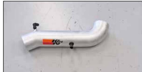
18. Remove the sealing O-ring from the sensor and then install the inlet air temperature sensor into the grommet installed into the intake tube.
