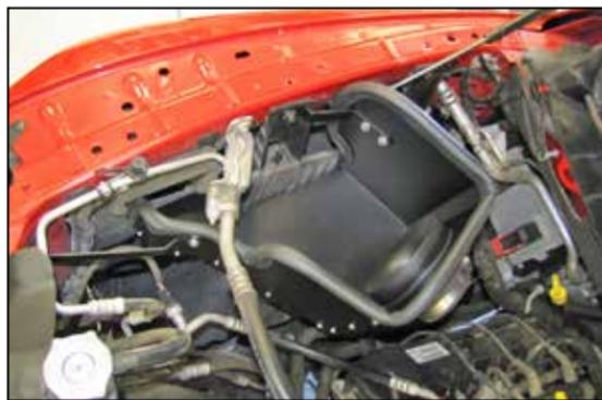
14. Install the heat shield into the vehicle and secure with the factory bolts removed in the previous steps.
