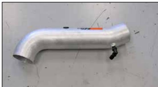
16. Install the 90° NPT fitting into the K&N® intake tube as shown.
