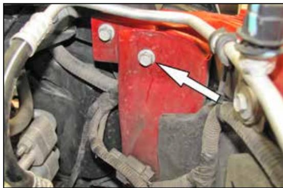
12. Remove the core support bolt shown.
