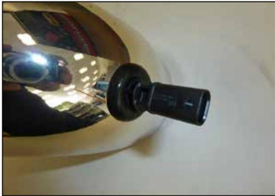
8. Install the provided grommet and factory temp sensor onto the K&N® intake tube.
