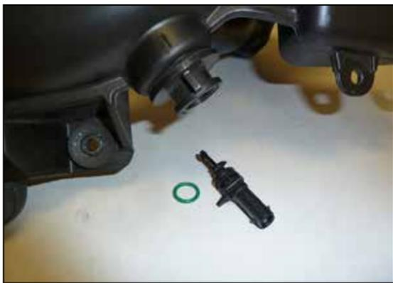
7. Remove the temp sensor from the factory intake tube by gently lifting the tab and rotating the sensor counter clockwise. Once the sensor is removed, remove the sealing O ring from the sensor.
