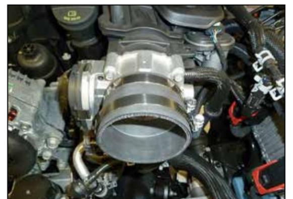
6. Install the provided coupler (08690) onto the throttle body and secure with the provided hose clamp.
