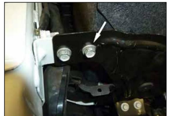
5. Remove the inner bolt that attaches fender bracket to the fender.
