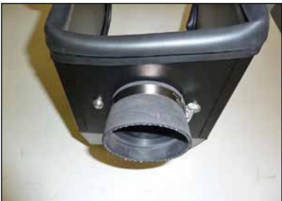
9. Install the air filter adapter onto the heat shield and secure with the provided hardware. Install the provided coupler (08186) onto the filter adapter and secure with the provided hose clamp.
