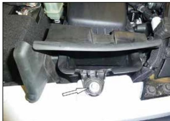
4. Remove the bolt shown that secures the fresh air intake duct to the fender, then lift and remove the complete intake system from the vehicle.
