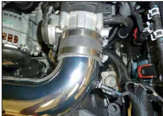
12. Install the intake tube into the coupler at the filter adapter and then into the coupler at the throttle body, adjust the tube for best fit and then secure with the provided hose clamps.
