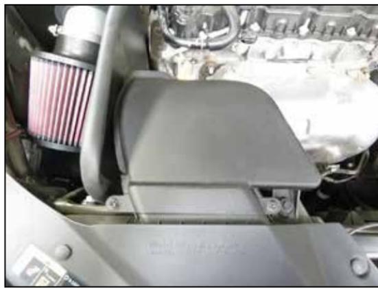
23. Reinstall the fresh air intake duct and secure with the factory hardware.
