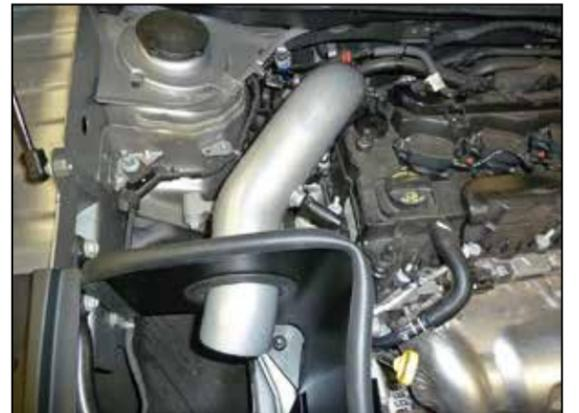
19. Install the K&N intake tube into the heat shield and then into the coupler, adjust the tube for best fit and then secure with the provided hose clamp.
