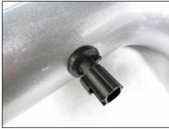
12. Install the IAT sensor into the grommet installed into the K&N intake tube.
