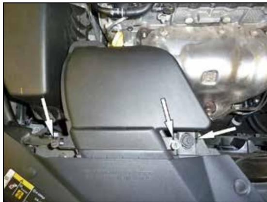
3. Remove the three bolts shown that secure the fresh air intake duct and then remove the duct from the engine.
