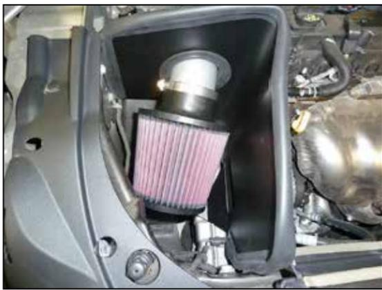
22. Install the K&N® air filter onto the intake tube and secure with the provided hose clamp.
