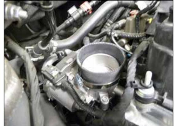
18. Install the provided coupler onto the throttle body and secure with the provided hose clamp.
