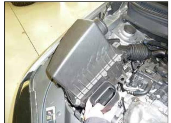
5. Pull the air filter housing straight up and remove it from the vehicle.
