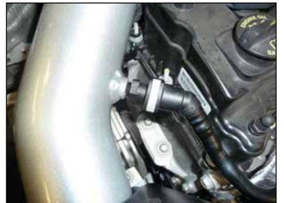
21. Reconnect the PCV to the Quick connect fitting installed into the K&N intake tube.
