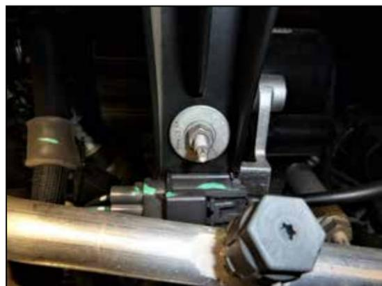
5. Remove the nut that secures intake plenum to the engine and then remove the intake plenum from the vehicle.
