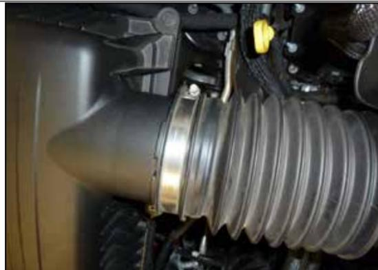
4. Loosen the clamp that secures the intake tube to the factory air filter housing.
