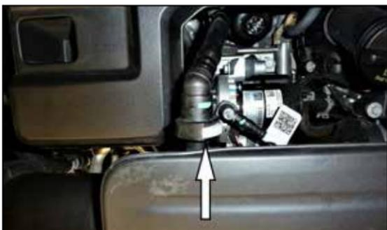
3. Depress the locking tab and then disconnect the CCV hose from the intake plenum.
