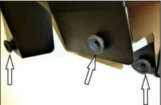
9. Remove the three mounting grommets from the factory air filter housing and install them into the heat shield as shown.
