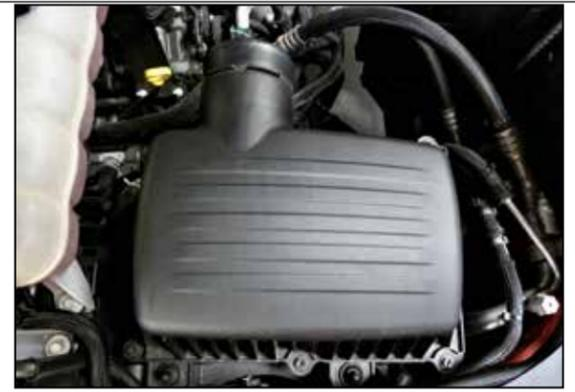
6. Pull the air filter housing straight up and remove it from the vehicle.
