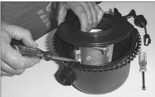
13. Using a flat blade screwdriver, push in and release the four clips that retain the mass air sensor retaining plate.
