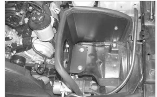
10. Install the heatshield as shown and secure with the provided hardware.
