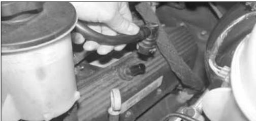
2. Rotate the crank case vent hose locking ring and pull the crank case vent hose off of the valve cover.
