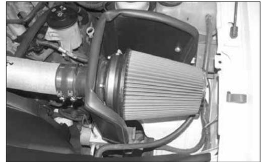
24. Install the K&N® air filter and secure with the provided hose clamp.
