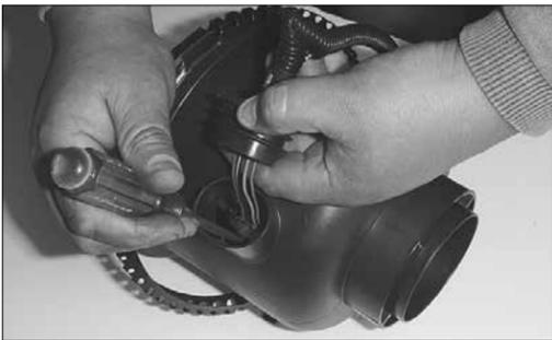
12. Slide the rubber grommet back and disconnect the primary mass air sensor electrical connection, using a flat blade screwdriver.
