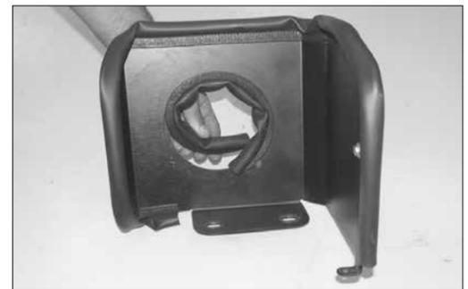
8. Install the edge trim into the hole in the heat shield as shown.
