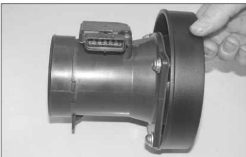
15. Attach the mass air adapter to the mass air sensor using the gasket and hardware provided as shown.
