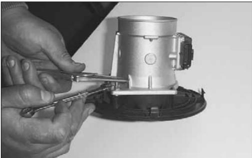
14. Using a pair of small vise grips or pliers, hold the stud while using a 10mm wrench to loosen the nuts, then remove the mass air sensor from the retaining plate.
