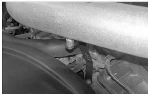
20. Attach the K&N® intake tube to the mounting bracket installed in step #17.
