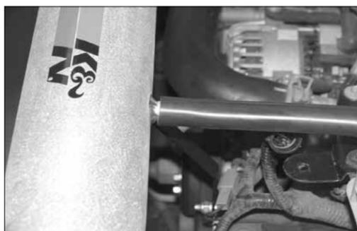
21. Install the provided silicone vent hose onto the valve cover and onto the K&N® intake tube as shown.
