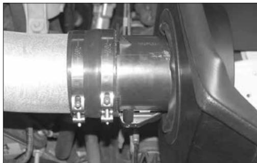
22. Install the mass air sensor assembly onto the K&N® intake tube and secure with the provided hose clamp.
