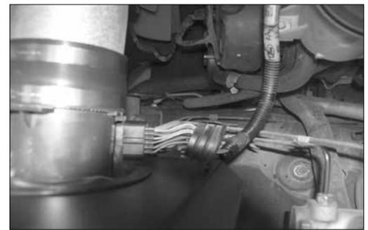
23. Reconnect the primary and secondary mass air sensor electrical connections.
