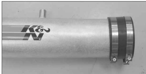
18. Install the silicone hose (08698) onto the K&N® intake tube and secure with the provided hose clamp as shown.
