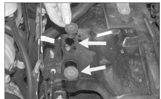
9. Install the provided nut inserts into the air box mounting holes as shown.
