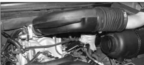
3. Loosen the stock intake tube hose clamps, and remove the intake tube from vehicle.
