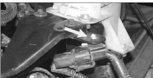
4. Unhook the secondary mass air sensor electrical connection from the power steering reservoir bracket, then unlock the electrical connection locking tabs and separate the electrical connection.
