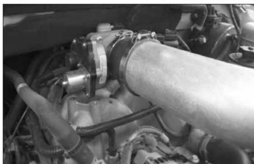
19. Install the K&N® intake tube into the silicone hose at the throttle body and secure with the provided hose clamp.
