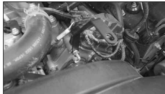
18. Install the tube mounting bracket (07198) onto the 8mm stud protruding from the engine with the factory nut, and the flat washer and wave washer provided. Do not completely tighten at this time.
