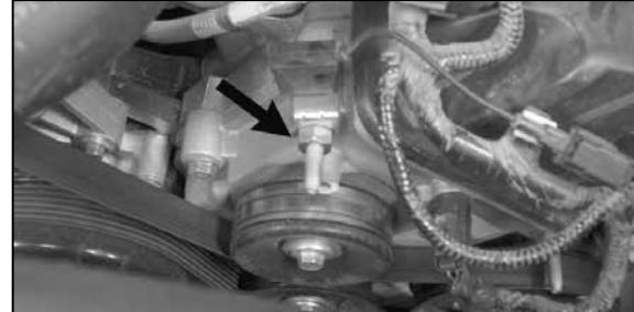
17. Remove the nut shown from the 8mm stud protruding from the engine.
