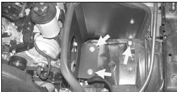
10. Install the heatshield as shown and secure with the provided hardware.
