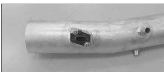
15. Install the mass air sensor assembly into the K&N® intake tube and secure with the factory mounting bolts.
