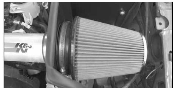
23. Install the filter assembly onto the K&N® intake tube and secure with the provided hose clamp.
