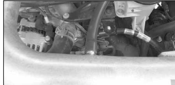
20. Install the provided silicone vent hose onto the valve cover and onto the K&N® intake tube as shown.
