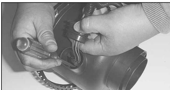
12. Slide the rubber grommet back and disconnect the primary mass air sensor electrical connection, using a flat blade screwdriver.
