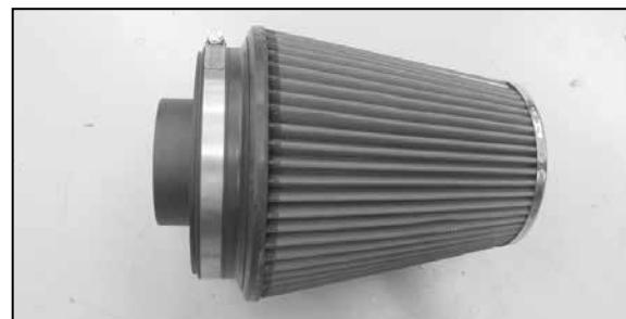
21. Install the filter adapter into the K&N® filter and secure with the provided hose clamp.
