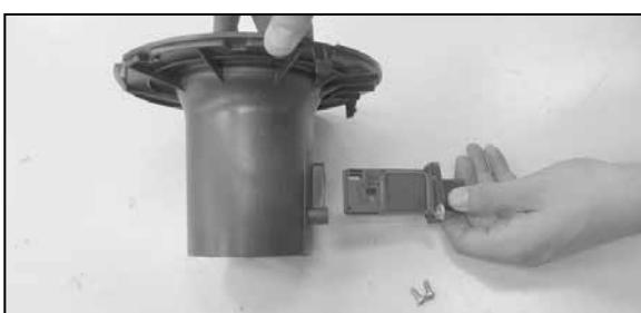
14. Remove the mass air sensor retaining screws and then remove the mass air sensors as shown.
