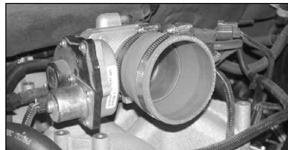
16. Install silicone hose (08724) onto the throttle body with the provided hose clamp as shown.
