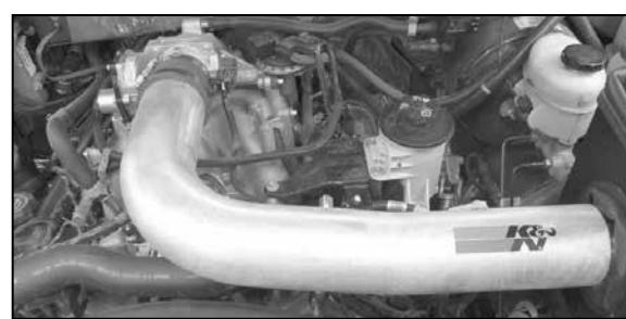
19. Install the K&N® intake tube into the silicone hose at the throttle body and align with the mounting bracket and secure with the provided hose clamp and hardware.
