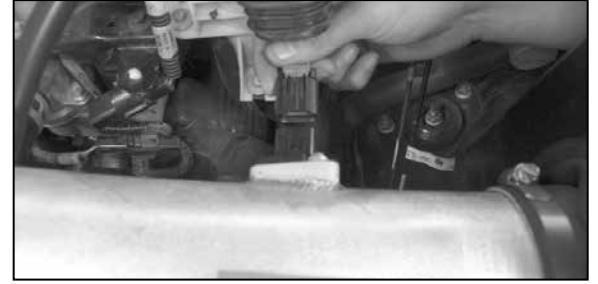
24. Reconnect the secondary mass air sensor electrical connection and then reconnect the mass air sensor primary electrical connection.
