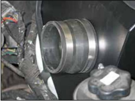
26. Install the provided silicone hose (08051) onto the filter adapter and secure with the provided hose clamp.
