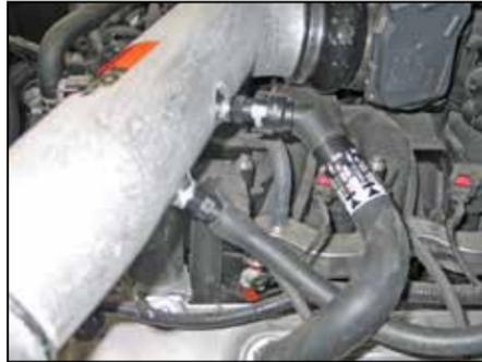
32. Connect the crankcase vent hose to the quick disconnect fitting. Attach the EVAP hose to the 1/2" hose barb.
