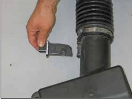
27. Remove the two screws securing the mass air sensor into the upper air box housing, then remove the mass air sensor from the housing.
