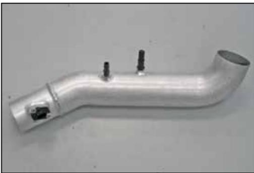
30. Install the 1/2" hose fitting into the K&N® intake tube as shown.
