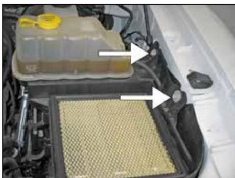
12. **NOTE: Be sure the engine is completely cooled before proceeding with this step.** Remove the two bolts that secure the lower air box/coolant reservoir to the inner fender. **NOTE: Some vehicles may be equipped with an alarm sensor that may need to be removed to gain access the rear most mounting bolts.**
