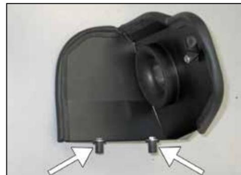
21. Install the provided nut inserts into the heat shield using the provided hardware.
