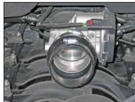
25. Install the provided silicone hose (084057) onto the throttle body and secure with provided hose clamp.
