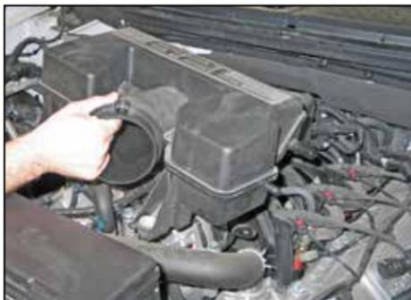
11. Remove the intake plenum from the vehicle.
