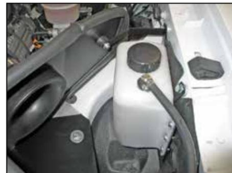
24. Route the coolant reservoir transfer hose to the coolant reservoir. Trim the hose for proper fit, then attach the hose onto the fitting and secure with the provided hose clamp.
