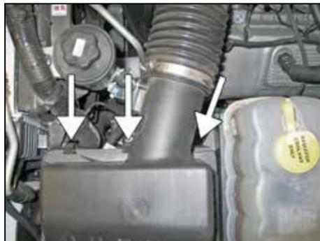
4. Release the three retaining clips on the upper air box.
