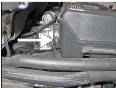
10. Loosen the hose clamp securing the intake plenum to the throttle body.
