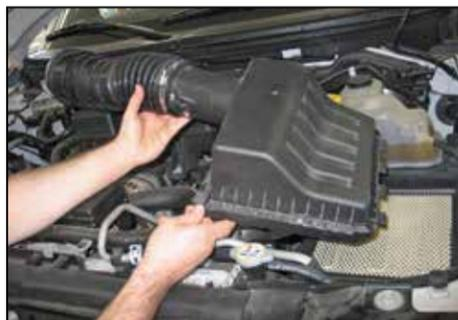
5. Remove the upper air box and intake tube assembly from the vehicle.
