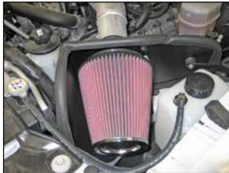
34. Mount the K&N® air filter onto the filter adapter and secure with a provided hose clamp. Transfer the coolant from the factory reservoir into the K&N® coolant reservoir.
