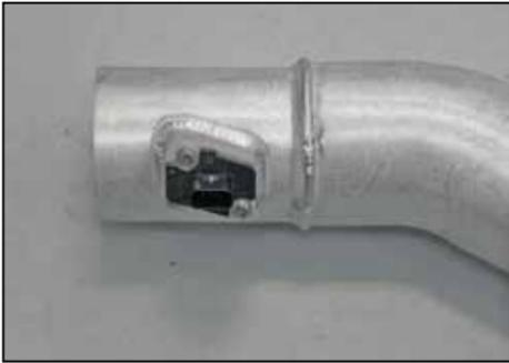
28. Install the mass air sensor into the K&N® intake tube and secure with the provided hardware.
