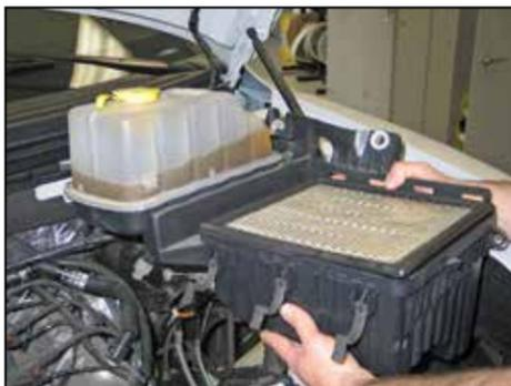
14. Remove the lower air box/coolant reservoir assembly from the vehicle.
