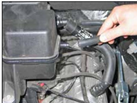
6. Disconnect the EVAP hose from the intake plenum.
