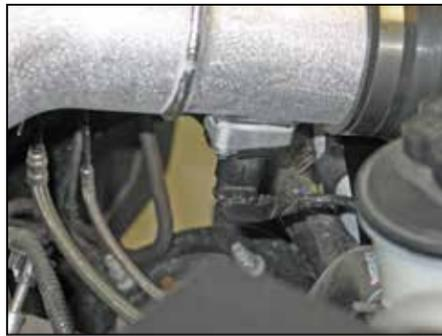
33. Connect the mass air sensor electrical connection.
