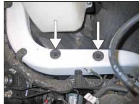
22. Remove the factory air box mounting grommets from the inner fender brace.
