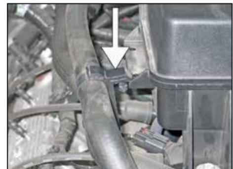
8. Unhook the heater hose retaining clip from the intake plenum.
