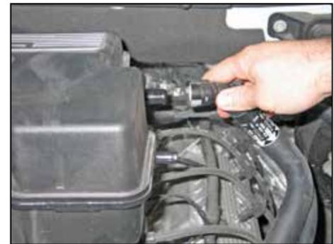
7. Release the locking tab and then disconnect the crankcase vent hose from the intake plenum.
