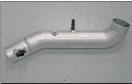
29. Install the provided quick disconnect fitting into the K&N® intake tube as shown.
