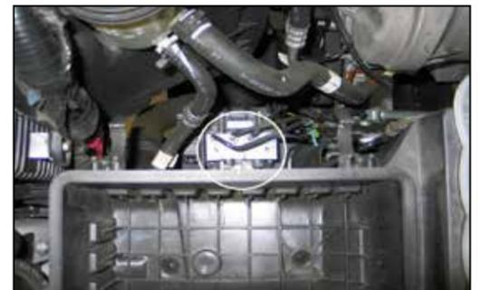
8. Remove the center upper airbox retaining clip from the lower airbox.
