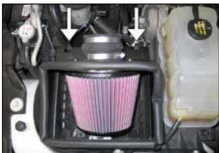
15. Install the completed heat shield/filter assembly onto the lower airbox. Secure with the two factory airbox retaining clips.
