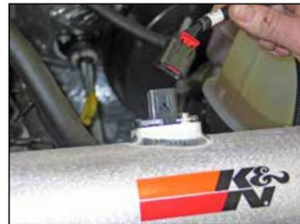
22. Connect the provided mass air sensor extension harness into the factory connector and then connect the open end to the mass air sensor electrical connection.
