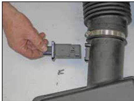
17. Remove the two screws securing the mass air sensor to the factory airbox, and then remove the mass air sensor.
