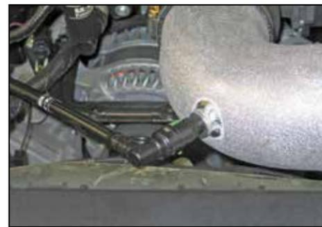
21. Rotate the crankcase vent coupler so it lines up with the fitting installed into the K&N® intake tube; connect the coupler to the fitting.
