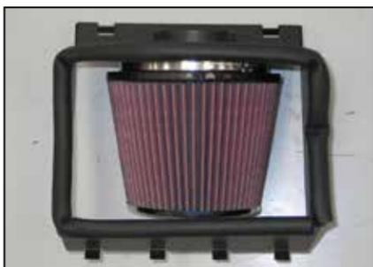
13. Install the K&N® air filter onto the filter adapter and secure with the provided hose clamp.
