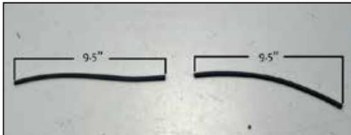
11. Cut the 19" section of small edge trim into two 9-1/2" lengths.
