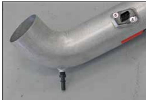
19. Install the provided crankcase vent fitting into the K&N® intake tube as shown.
