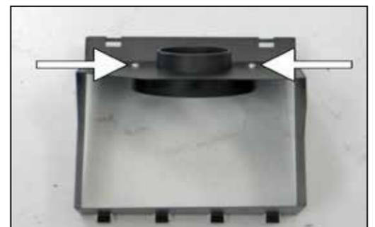
9. Install the K&N® filter adapter into the heat shield as shown. Secure with the provided hardware.
