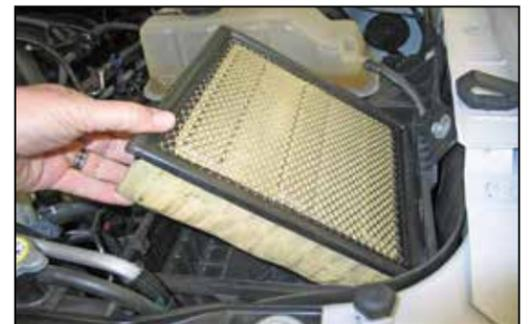
7. Remove the air filter from the lower airbox.
