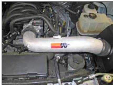
20. Install the K&N® intake tube; insert the lower end into the silicone hose attached to the heat shield /air filter assembly. Attach the upper end of the intake tube to the silicone hose secured to the throttle body. Secure the intake tube with the provided hose clamps.
