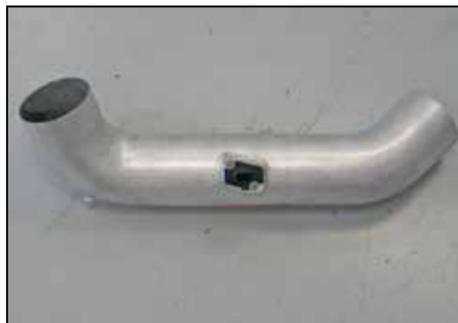
18. Install the mass air sensor into the K&N® intake tube as shown, secure with the provided hardware.
