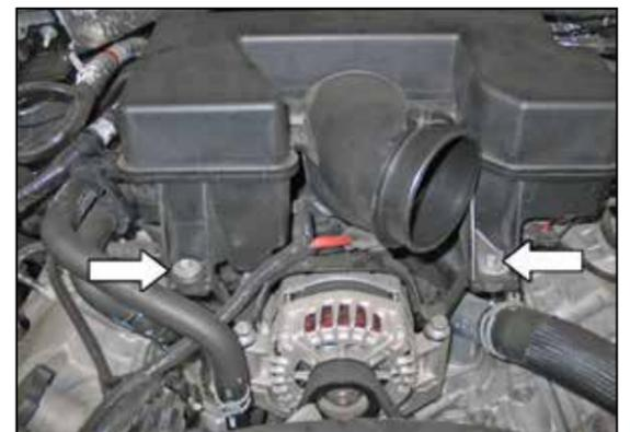
7. Remove the two bolts securing the intake plenum to the intake manifold and then loosen the hose clamp securing the plenum to the throttle body.
