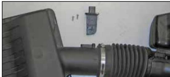
17. Remove the mass air sensor from the factory air box.
