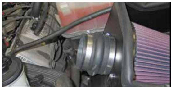
15. Install the provided silicone hump hose (5-576) onto the filter adapter and secure with the provided hose clamp.
