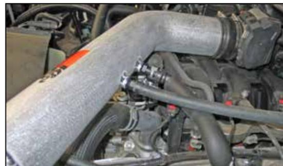
20. Connect the crank case vent hose and EVAP vent hose to the K&N® intake tube.
