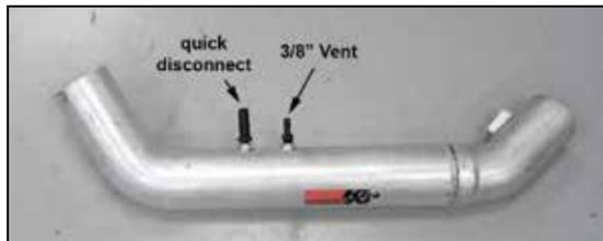
16. Install the quick disconnect and 3/8 NPT vent fittings into K&N® intake tube as shown.
