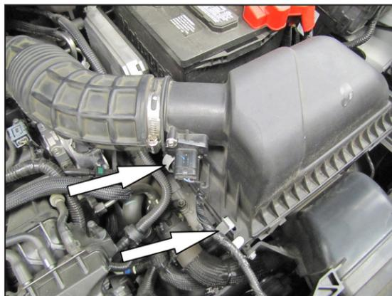
3. Disconnect the inlet air temperature sensor electrical connection and unhook the harness from the air box.
