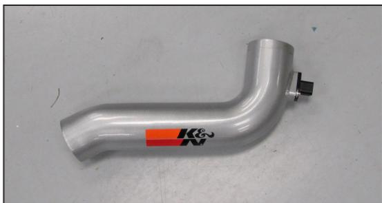
15. Install the inlet air temperature sensor into the K&N® intake tube and secure with the hardware provided.
