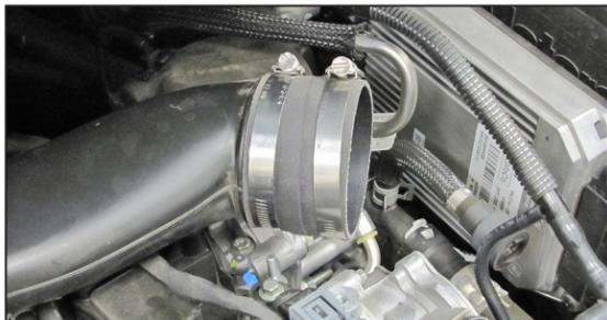
13. Install the provided coupling hose (08711) onto the turbo inlet tube and secure with the provided hose clamp.
