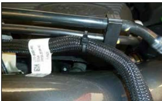
16. Secure the coolant hose using the provided tie wrap.
