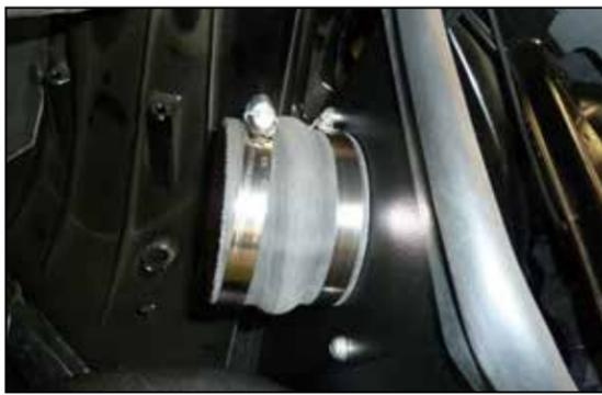
13. Install the hump coupler onto the filter adapter and secure with the provided hose clamp.
