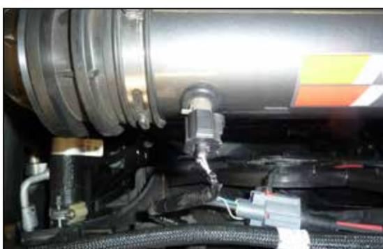
17. Reconnect the inlet temperature sensor electrical connection.
