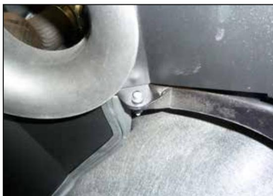
11. Secure the lower front heat shield tab with the hardware provided.
