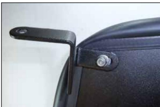
8. Install the provided bracket onto the heat shield as shown using the provided hardware.
