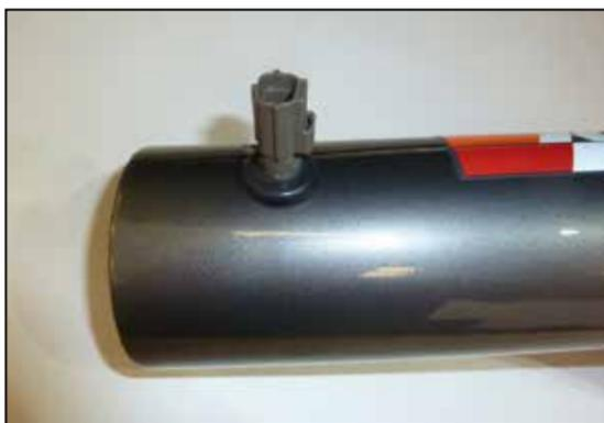
14. Remove the inlet air temperature sensor from the factory air filter housing, remove the O-ring and then install it into the K&N intake tube using the provided grommet.
