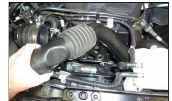
5. Release the two tabs that secure the fresh air duct to the inlet in the core support and remove the fresh air duct.
