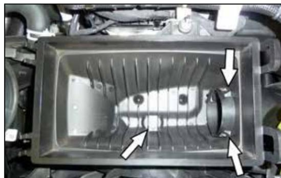
4. Remove the mounting nut securing the lower air filter housing, release the tabs securing the fresh air inlet duct and then remove the lower housing.
