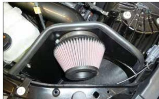
18. Install the K&N air filter and secure with the provided hose clamp.
