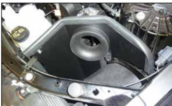
9. Install the heat shield into the vehicle as shown.
