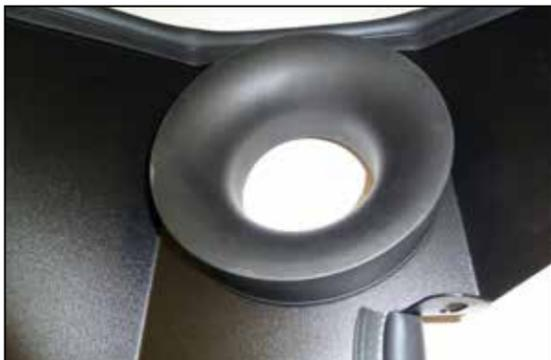
7. Install the filter adapter into the heat shield and secure with the provided hardware.
