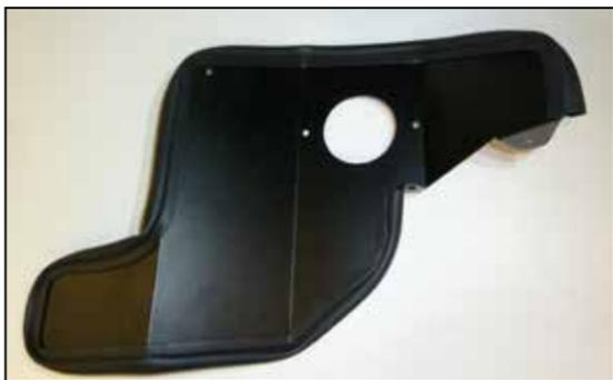
6. Install the provided edge trim onto the heat shield as shown, some trimming of the edge trim will be necessary.
