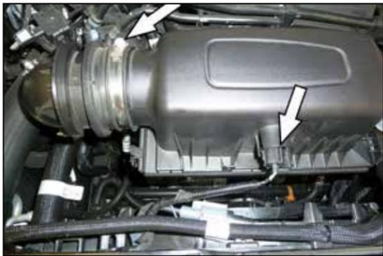
2. Loosen the hose clamp that secures the intake hose to the air filter housing and disconnect the hose from the housing. Disconnect the inlet air temperature sensor electrical connection
