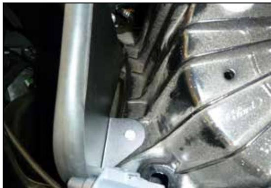
10. Secure the rear mount of the heat shield near the strut tower with the hardware provided.
