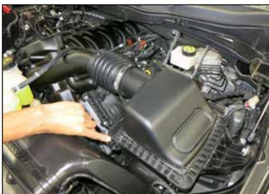
2. Release the two locking tabs that secure the upper air filter housing.
