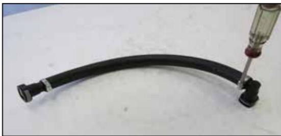
7. Assemble the provided CCV hose assembly using the hose, fittings, and clamps.
