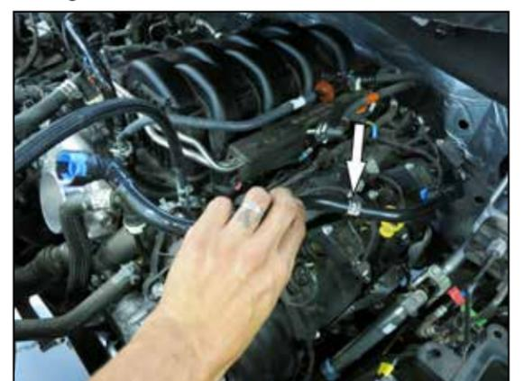
6. Disconnect the CCV line from valve cover.
