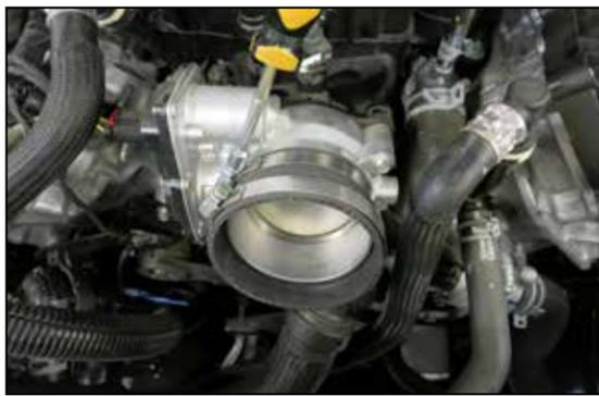
13. Install the provided straight coupler onto the throttle body and secure with the provided hose clamp.
