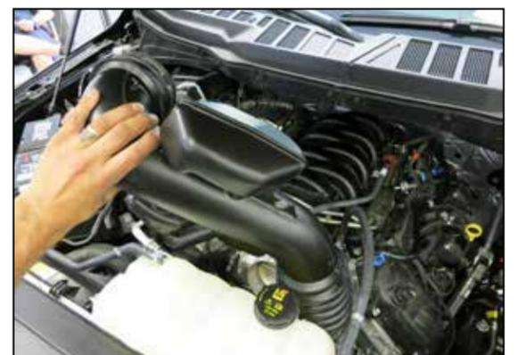
5. Remove the intake tube and upper air filter housing from the vehicle.
