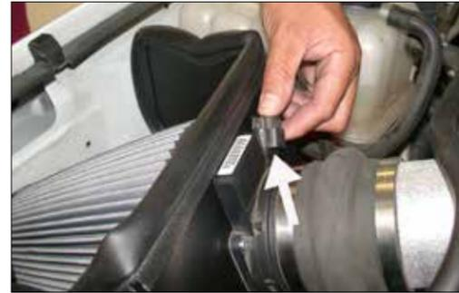
19. Reconnect the mass air sensor electrical connection as shown.
