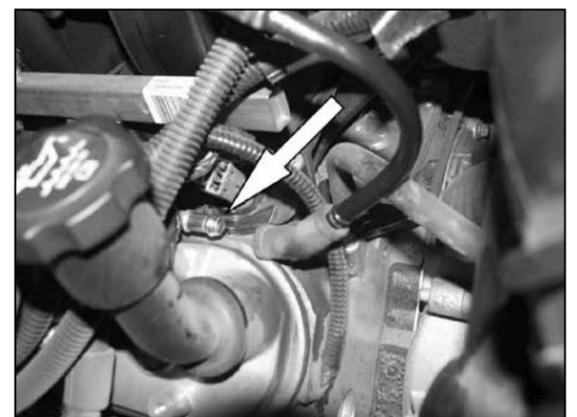
5. Disconnect crankcase vent hose from the valve cover as shown.
