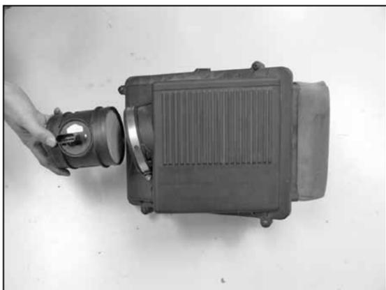
8. Loosen the hose clamp and remove the mass air sensor from the air cleaner as shown.
