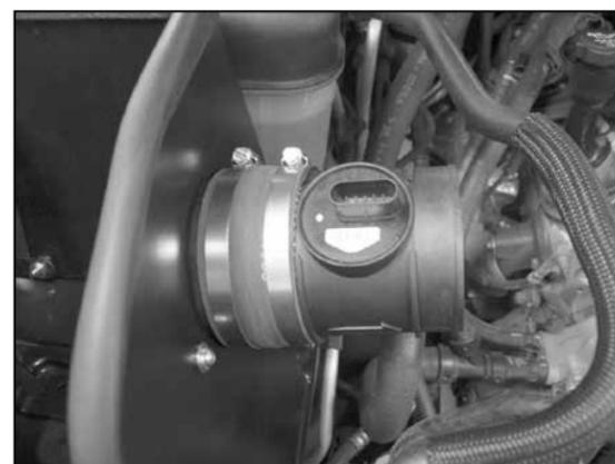
18. Install the mass air sensor assembly into the silicone hose on the filter adapter and secure with provided hose clamp.
