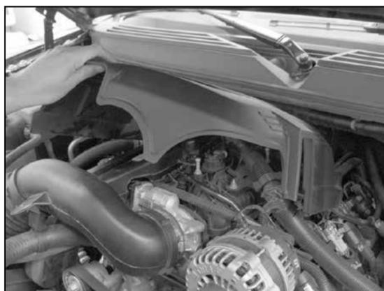
3. Lift up on the front of the engine cover to disengage from the mounting grommets. Then pull forward and remove the engine cover from the engine as shown.
