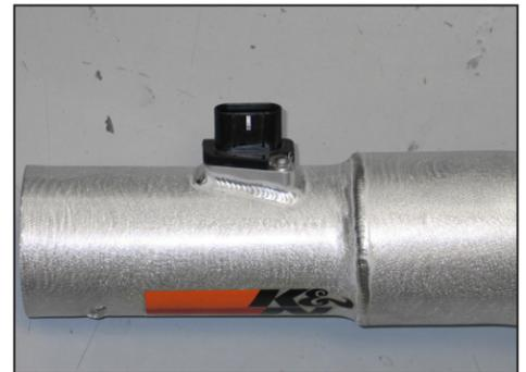
Install the mass air sensor into the K&N® intake tube and secure with the provided hardware.
