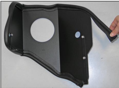
10. Install the long edge trim onto the heat shield as shown.
