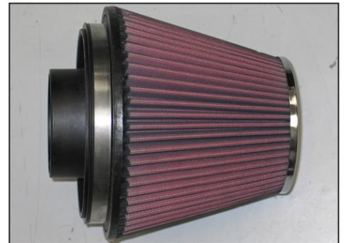
22. Install the air filter adapter into the K&N® air filter and secure with the provided hose clamp.
