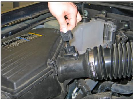
2. Depress the locking clip on the mass air sensor electrical connection, then separate the mass air sensor electrical connection.
