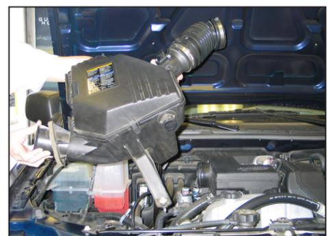
6. Lift the air box up, removing it from the vehicle as shown.
