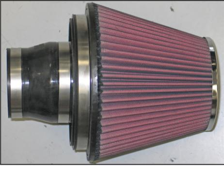
23. Install silicone hose (08724) onto the air filter adapter and secure with the provided hose clamp.
