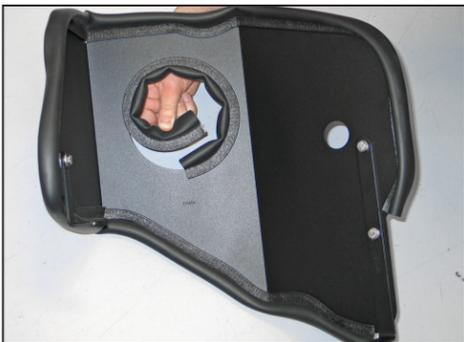
11. Install the small edge trim into the heat shield hole as shown.
