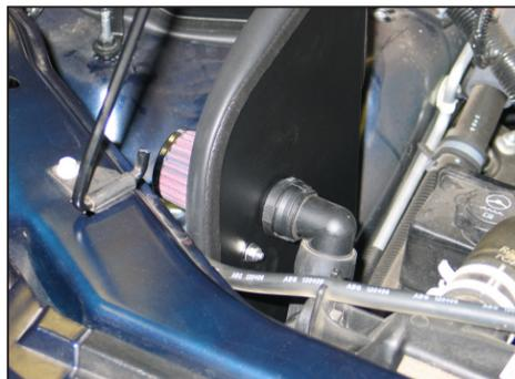
15. Secure the air pump fresh air tube to the adapter as shown.
