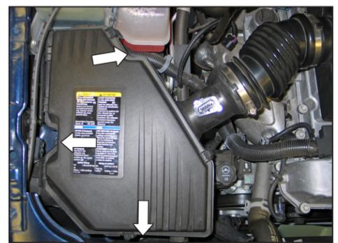
5. Loosen the single retaining nut and two air box retaining bolts.
