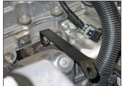
16. Install the tube mounting bracket (06495) onto the cylinder head as shown. Secure with the provided hardware.
