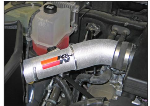
21. Install the K&N® intake tube into the silicone hose at the throttle body and align it with the tube mounting bracket installed in step 16. Secure with the provided hardware and hose clamp.
