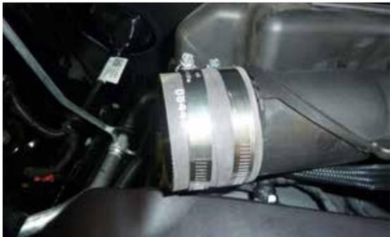
8. Install the provided straight coupler onto the intake plenum and secure with the provided hose clamp.
