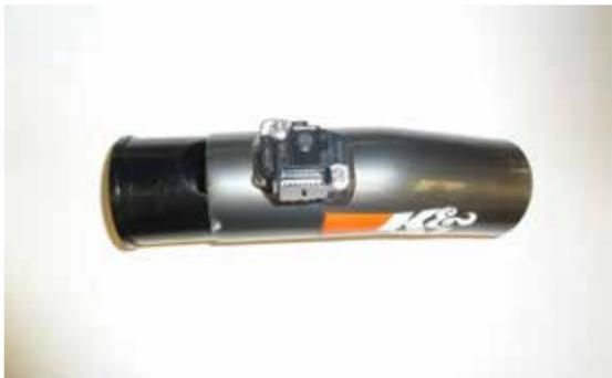
10. Install the maf sleeve into the K&N intake tube so the lip on the end of the sleeve stops against the end of the intake tube.
