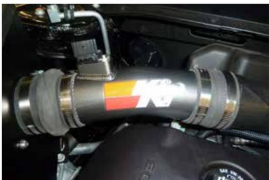
11. Install the intake tube into the hump coupler and then into the straight coupler, adjust the tube for best fit and then secure with the provided hose clamp.
