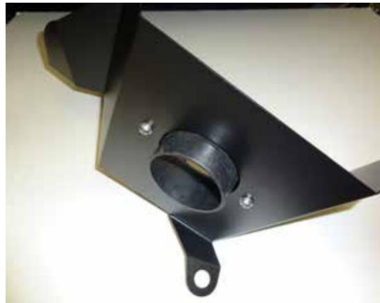
3. Install the radius filter adapter into the heat shield and secure with the provided hardware.
