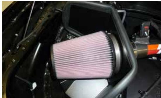
13. Install the K&N air filter onto the intake tube and secure with the provided hose clamp.
