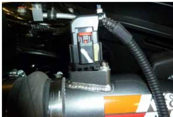
12. Reconnect the mass air sensor electrical connection.
