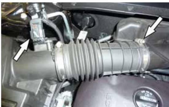
2. Disconnect the mass air sensor electrical connection and loosen the hose clamp that secures the intake hose to the plenum. Pull straight up and remove the complete air filter housing assembly from the vehicle. **NOTE: K&N Engineering, Inc., recommends that customers do not discard factory air intake**
