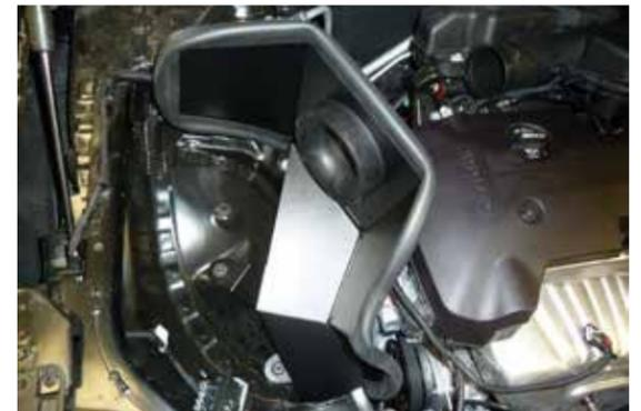
6. Install the heat shield assembly onto the mounting studs as shown.
