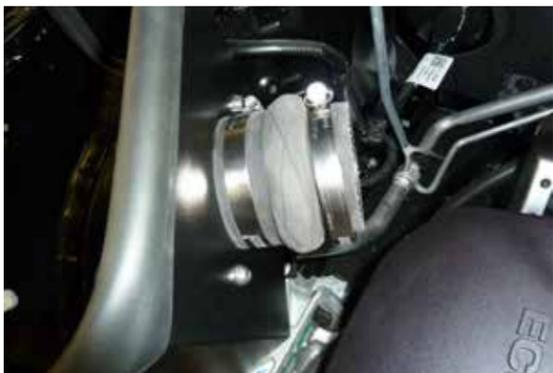
7. Install the provided hump coupler onto the filter adapter and secure with the provided hose clamp.
