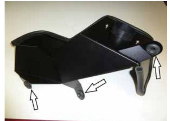
5. Remove the three factory mounting grommets from the factory air filter housing and install them into the K&N heat shield as shown.
