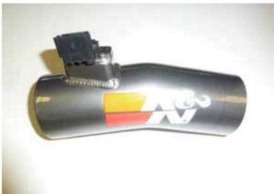
9. Remove the mass air sensor from the factory housing and install it into the K&N intake tube using the provided hardware.
