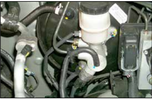
9a. On four wheel drive vehicles, secure the front differential vent tube to the front brake hardline as shown with the provided tie wrap.
