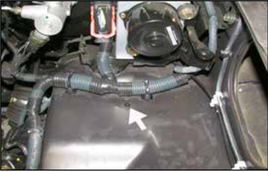
10. From underneath the inner fender panel remove the plastic rivet as shown.
