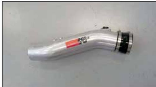
21. Install the provided silicone hose (08051) onto the K&N® intake tube as shown and secure with the provided hose clamp.
