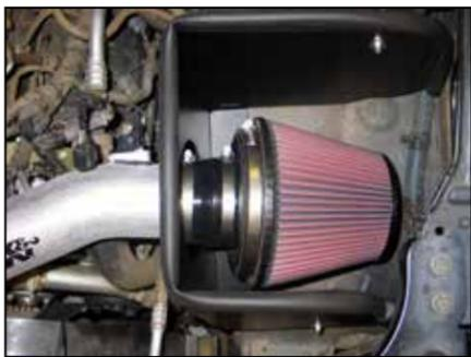
28. Install the filter assembly onto the K&N® intake tube and secure with the provided hose clamp.
