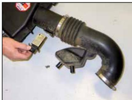
19. Remove the mass air sensor from the stock intake tube as shown.
