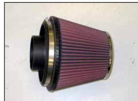
27. Install the filter adapter into the K&N® air filter and secure with the provided hose clamp.
