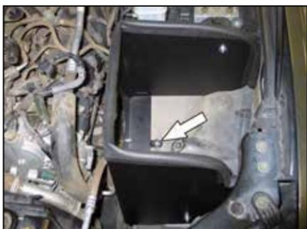
15. Install the heat shield assembly into position and secure with the provided hardware and the bolt removed in the previous step.
