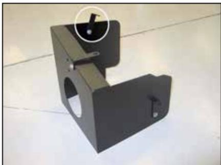
12. Install the heat shield mounting bracket (070632) onto the heat shield as shown using the provided hardware.
