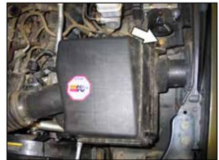
7. Remove the bolt shown which secures the airbox to the inner fender.
