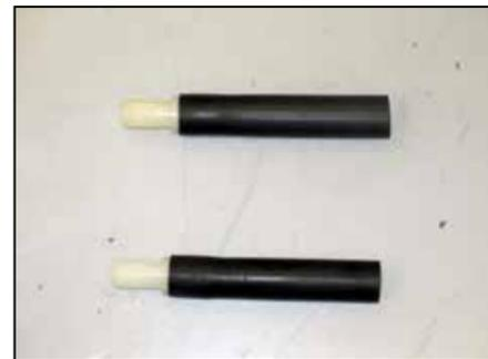
23. Install the two provided hose menders into the each of the crankcase vent hose sections as shown.
