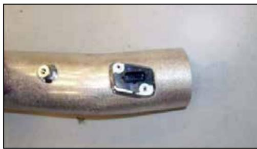
20. Install the mass air sensor into the K&N® intake tube and secure with the provided hardware.
