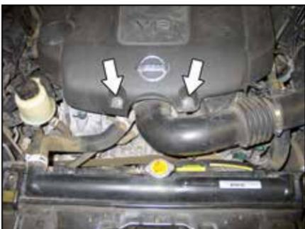
3. Remove the two bolts which secure the engine cover to the engine.
