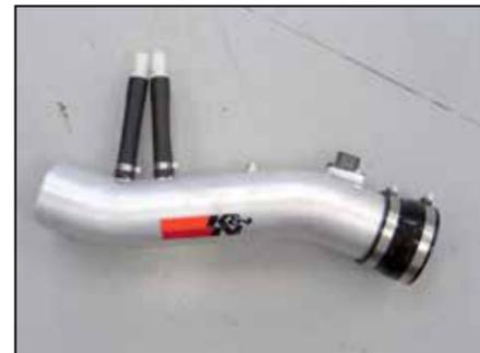
25. Attach the two modified crankcase hoses onto the 1/4 NPT fittings.
