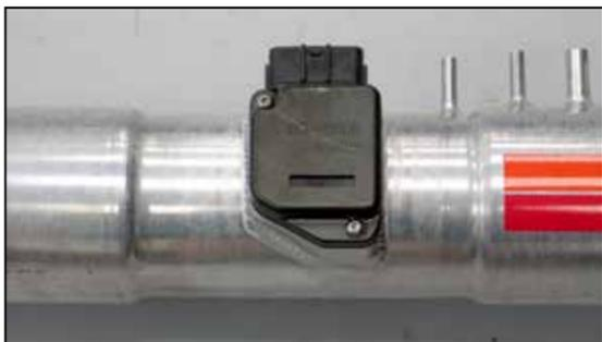
10. Install the mass-air sensor into the K&N® intake tube, and secure with the provided screws as shown.
