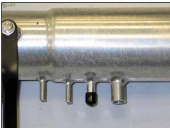
19. On vehicles that are not equipped with the 4th vacuum line, install the provided plug onto the vent tube as shown.
