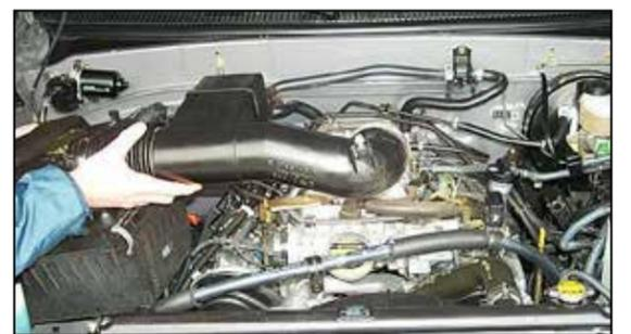
8. Remove the complete air induction system.
