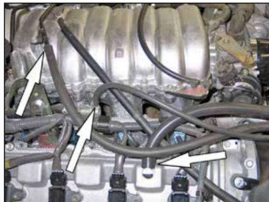
22. Replace the crank case vent line, EVAP vent line, and fuel pressure vent line with vent lines supplied.
