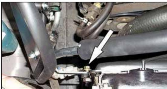
16. Secure the upper bracket to the fan shroud with the original bolt.
