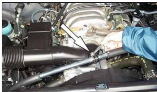
4. Loosen and remove the bolt that secures the AC line to the stock intake tube.
