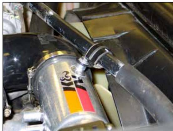
21. Reconnect the A/C line to the K&N® intake tube using the original bolt removed in step #4.
