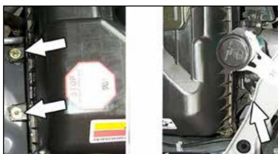
6. Loosen the three bolts that secure the air box assembly.
