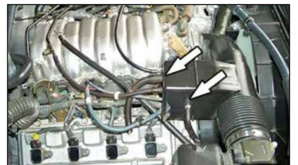
7. Disconnect the four rubber hoses from the engine as shown by the arrows.
