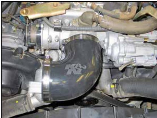
17. Install the provided silicone hose (084095) onto the throttle body with the provided hose clamps.
