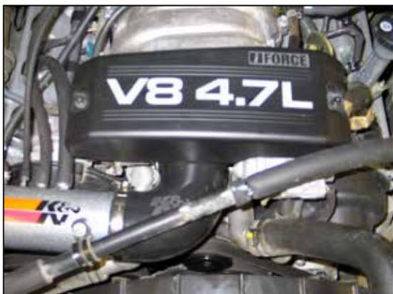
27. Reinstall the throttle body cover and secure with the original nuts.
