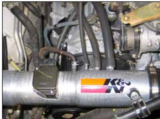
23. Install the one factory P/S vent line, crank case vent line, EVAP vent line, and fuel pressure vent line onto the K&N® intake as shown.
