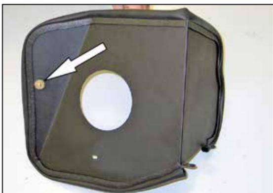
12. Install the rubber mounted stud onto the heat shield as shown with the provided hardware.
