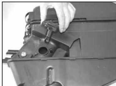
18. Remove the two screws that secure the mass air sensor to the air box assembly, then remove the mass air sensor as shown.
