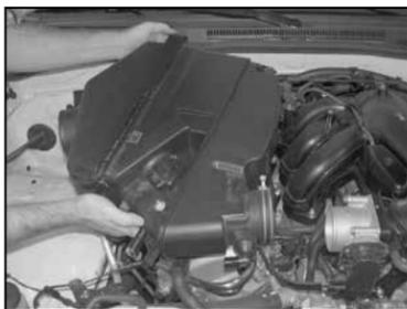
11. Remove the air box assembly from the engine as shown.
