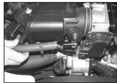
8. Remove the crank case vent hose from the air box as shown.
