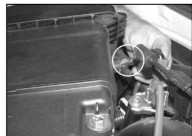
9. Remove the fuel pressure regulator hose from the back side of the air box.
