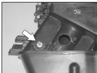
20. Using a 4mm socket, remove the engine cover mounting stud from the stock air box.
