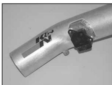
19. Install the mass air sensor into the K&N® intake tube as shown using the provided hardware.
