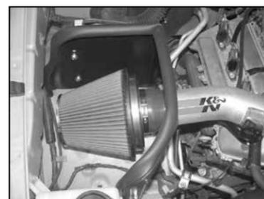
28. Install the K&N® air filter onto the intake tube as shown.
