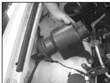
6. Remove the two bolts that secure the resonator to the inner fender, then remove the resonator from the vehicle as shown.
