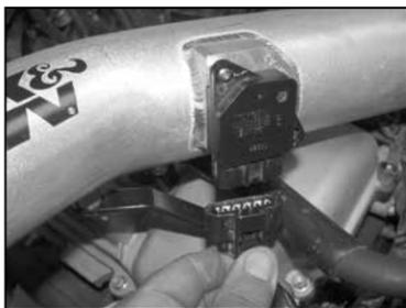
29. Reconnect the mass air sensor electrical connection.
