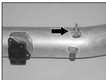
21. Install the engine cover-mounting stud into the K&N® intake tube as shown.
