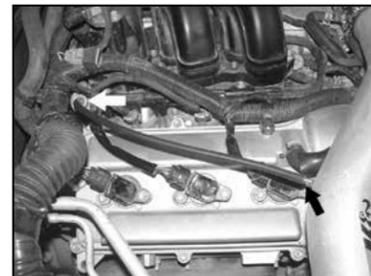
24. Remove the stock vacuum hose from the fuel pressure regulator. Install the provided silicone hose onto the fuel pressure regulator and then attach the opposite end to the K&N® intake tube.
