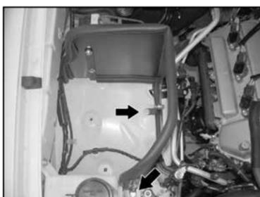
16. Install the heat shield onto the vehicle and secure with the provided hardware and the nut removed in step #15.
