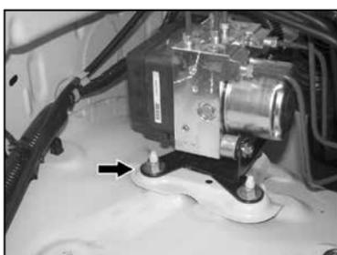
15. Remove the ABS pump mounting nut shown.
