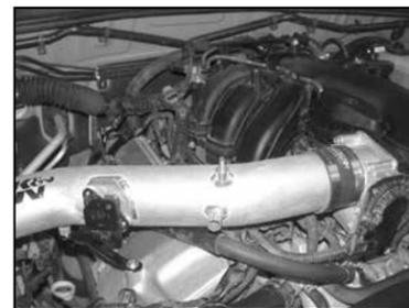
23. Install the K&N® intake tube assembly onto the throttle body and align the tube-mounting bracket with the threaded boss on the valve cover; secure with the provided hardware as shown.
