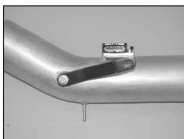
22. Install the provided tube-mounting bracket onto the K&N® intake tube with the provided hardware as shown.
