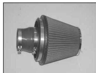
27. Install the provided silicone hose (084055) onto the air filter assembly and secure with the provided hose clamp as shown.
