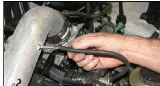
20. Install the provided vacuum hose onto the fuel pressure regulator and then onto the K&N intake tube as shown.
