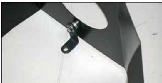
9. Install the small heat shield mounting bracket (070812A) with the provided spacer onto the heat shield as shown.
