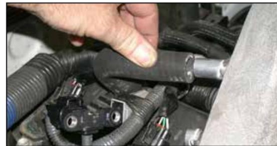
Install the provided crank case vent hose onto the valve cover port and then onto the K&N intake tube and secure with the provided hose clamps.
