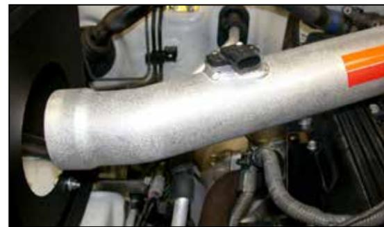
19. Secure the K&N intake tube to the tube mounting bracket with the provided hardware and then tighten the hose clamp at the throttle body.
