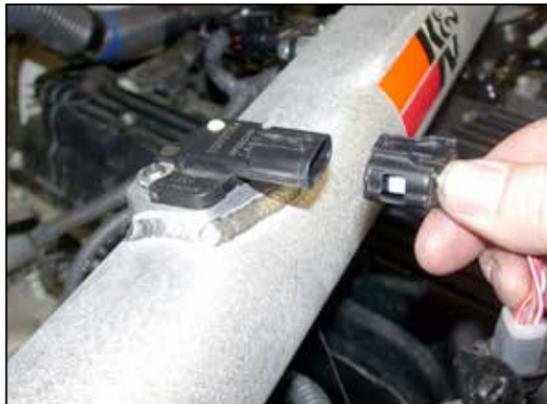
27. Reconnect the mass air sensor electrical connection as shown.
