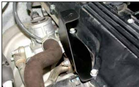
14. Install the tube mounting bracket assembly onto the valve cover using the factory bolts removed in step #13.
