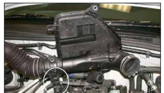
6. Disconnect the wire harness-retaining clip shown from the intake plenum.
