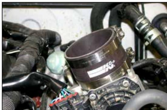
15. Install the provided silicone hose (08440) onto the throttle body and secure with the provided hose clamp.
