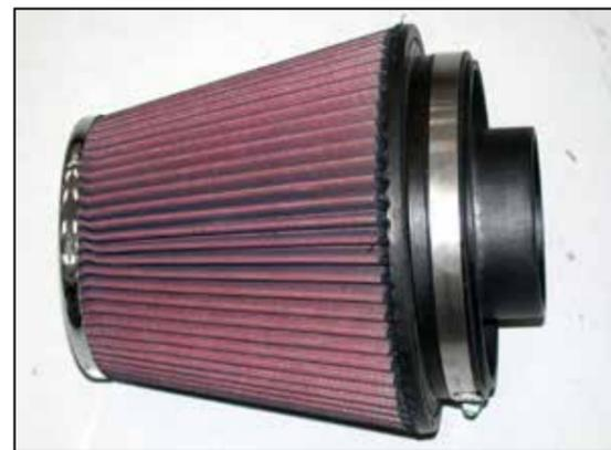
23. Install the radius filter adapter into the K&N air filter and secure with the provided hardware as shown.
