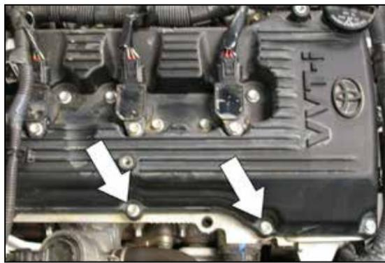
13. Remove the two valve cover bolts shown.
