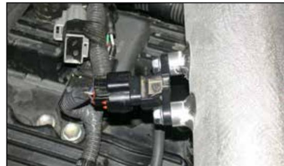
22. Install the pressure sensor onto the K&N intake tube using the bolts removed in step #3.
