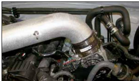
18. Install the K&N intake tube onto the throttle body and align with the tube mounting bracket that was installed in step #14.
