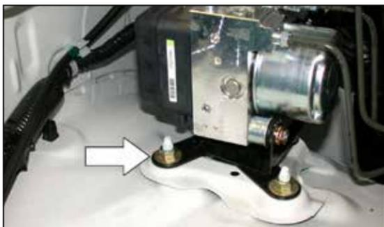
11. Remove the ABS pump mounting nut shown.
