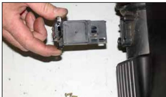
16. Remove the two mass air sensor retaining screws and then remove the mass air sensor from the factory air box.
