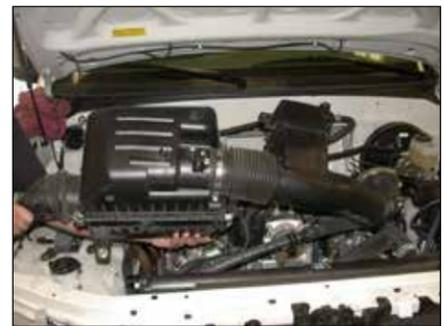
8. Remove the complete intake assembly from the vehicle as shown.
