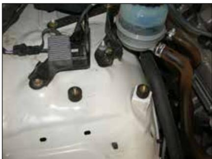
14. Install the two rubber mounted studs to the original air box mounting holes as shown.
