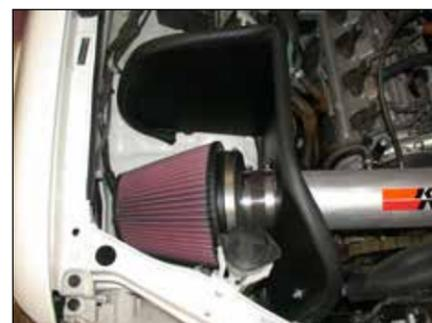
27. Install the air filter assembly onto the K&N® intake tube and secure with the provided hose clamp.
