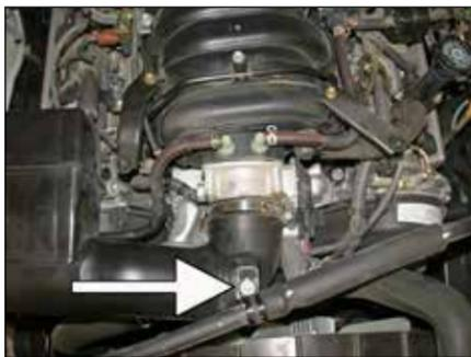
4. Loosen and remove the bolt that secures the A/C hose to the stock intake tube.
