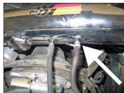
24. Attach the power steering pressure switch vent hose to the K&N® intake tube as shown.
