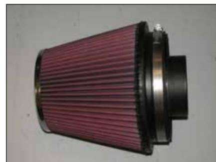
25. Install the filter adapter into the air filter as shown and secure with the provided hose clamp.
