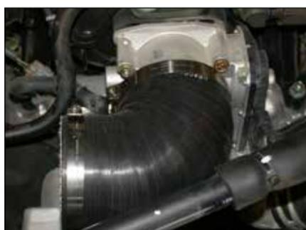
18. Install the silicone hose (084088) onto the throttle body and secure with the provided hose clamp as shown.
