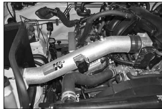
21. Install the K&N® intake tube into the silicone hose at the throttle body and align the mounting stand off with the bracket installed in step #20. Secure the intake tube with the hose clamp and hardware provided.
