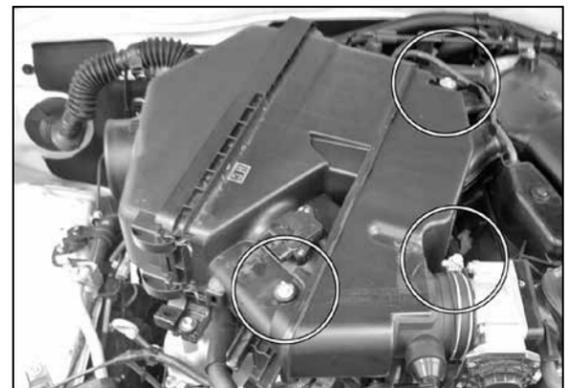
9. Loosen the hose clamp at throttle body, then remove the two bolts that secure air box to engine.
