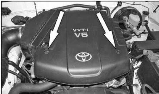
2. Loosen the two nuts that secure the engine cover, and then remove the engine cover from the engine.
