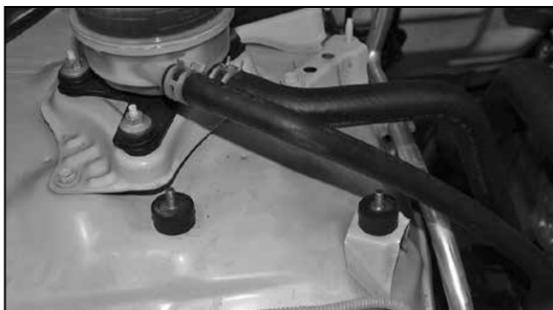
14. Install the two remaining rubber mounted studs to the original air box mounting holes as shown.
