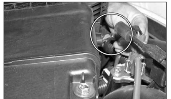
8. Remove fuel pressure regulator hose from back side of air box.
