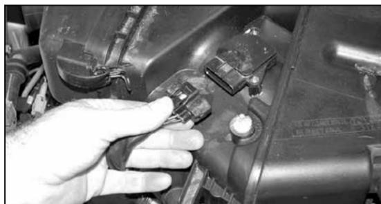
6. Disconnect the two mass air wire harness retaining clips from air box, then disconnect the mass air sensor electrical connection.
