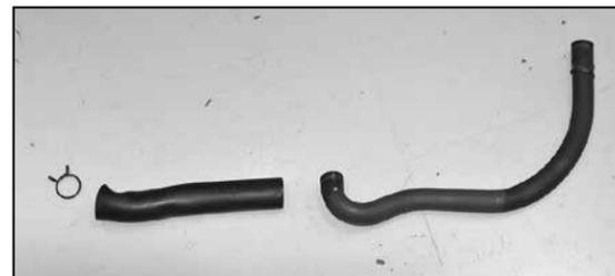
22. Remove the crank case vent hose from the valve cover and then remove the factory clamp and outer cover from the crank case vent hose as shown.
