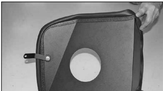
13. Secure the mounting bracket to the rubber mounted studs to the original air box mounting holes as shown.
