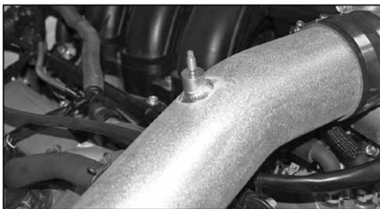
30. Install the engine cover mounting stud into the threaded stand off on the K&N® intake tube as shown.
