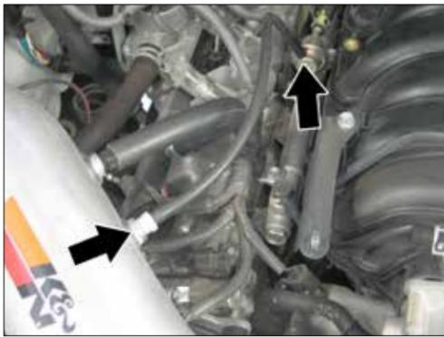
26. Install the provided fuel pressure hose onto the fuel pressure regulator and then connect the open end onto the remaining NPT fitting installed into the K&N® intake tube as shown.
