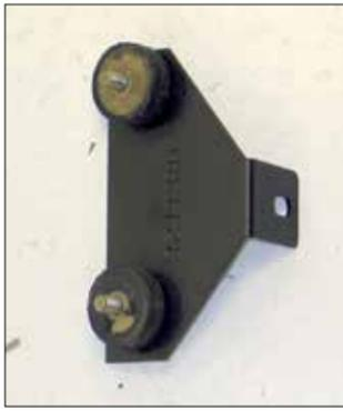
14. Secure the provided rubber mounted studs to the tube mounting bracket as shown using the provided hardware.
