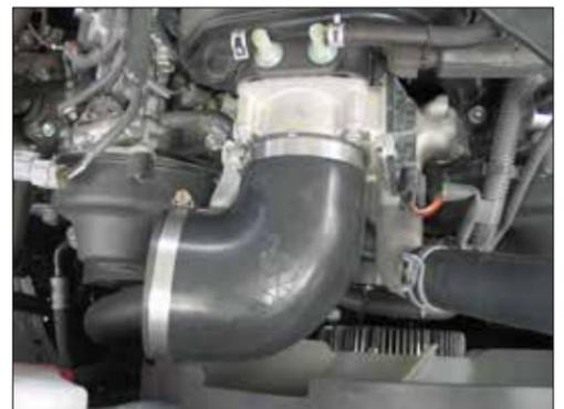
20. Install the silicone hose (#084086) onto the throttle body and secure with the provided hose clamp.
