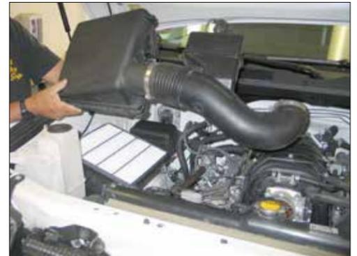
6. Release the four upper air box clam shell clamps, then remove the upper airbox and intake tube assembly.
