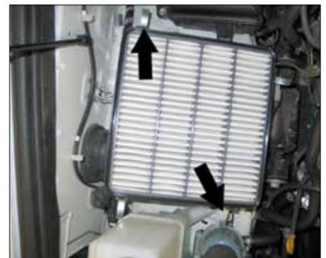
7. Remove the two factory bolts that secure the lower air box to the inner fender.
