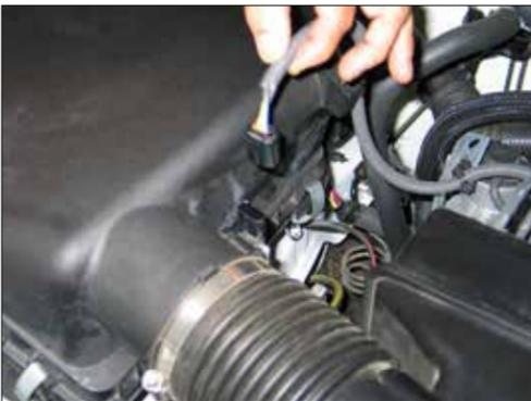
2. Disconnect the mass air sensor electrical connection. Then unclip the mass air sensor wiring harness from the air box.
