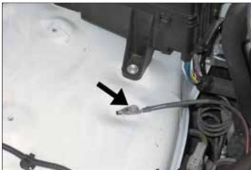
16. Remove the bolt that retains the ground strap to the inner fender.
