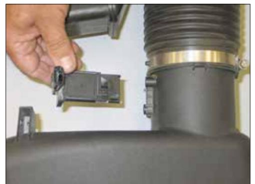
21. Remove the factory screws that secure the mass air sensor to the factory intake tube, and then remove the mass air sensor from the stock intake tube.
