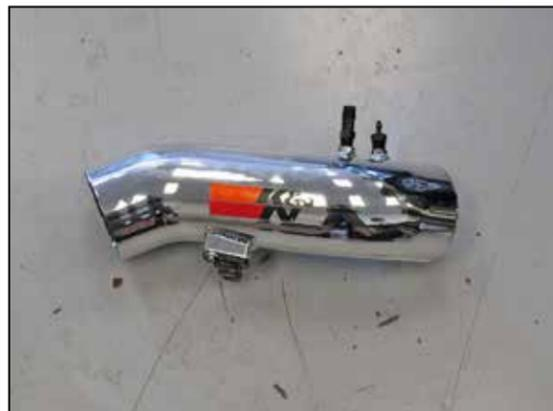
18. Install the provided NPT vent fittings into the K&N® intake tube as shown.
