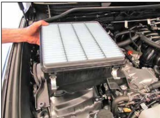
7. Loosen the three bolts securing the lower air box and then remove the lower air box from the vehicle.
