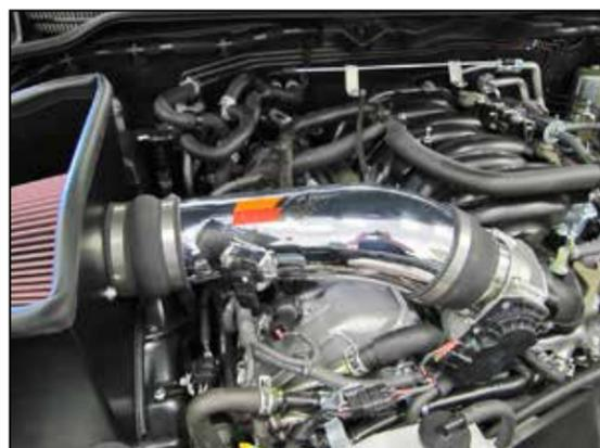
20. Install the K&N® intake tube into the hump coupler at the heat shield and then into the coupler at the throttle body, adjust the tube for best fit and then secure with the provided hose clamp.
