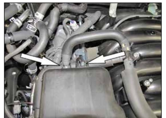
5. Disconnect the crank case vent hose and fuel pressure line from the intake resonator.
