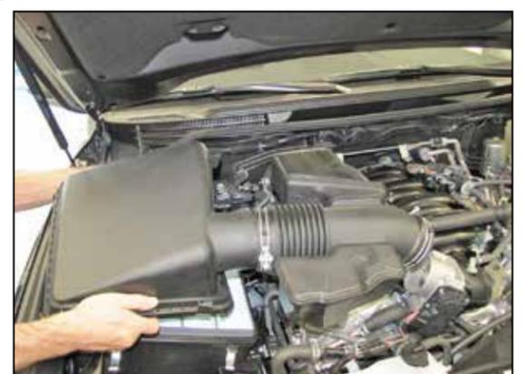
6. Release the four retaining clips securing the upper air box and then remove the upper air box and intake tube assembly from the vehicle.
