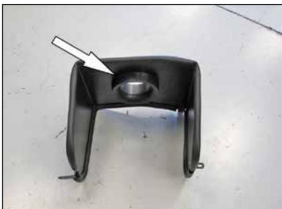
11. Install the filter adapter onto the heat shield and secure with the provided hardware.
