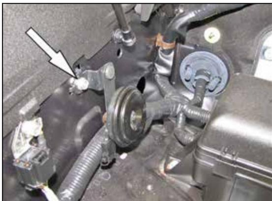
12. Remove the bolt which secures the horn to the inner fender.
