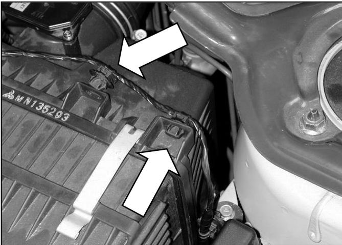
e. Unclip the Mass Air Flow (MAF) sensor wiring harness from the air filter housing. These clips can be removed undamaged from the harness using a small flat head screwdriver.
