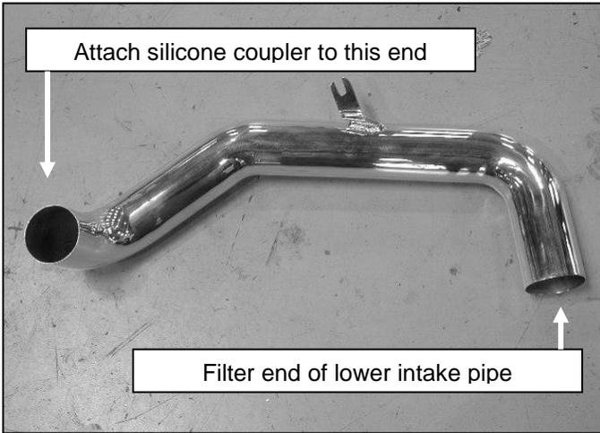
e. Ensure that the inside of the lower intake pipe and air filter are clean and free from any foreign objects and/or obstructions. Install the 2.75" silicone coupler over the end of the pipe using the 2.75" hose clamp.
