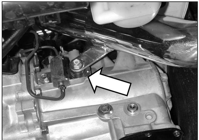
h. Align the intake mounting bracket with the rubber mount installed in step 3b. Secure using the supplied washer and nylok nut. Be sure that the bracket and intake do not contact the clutch lines or slave cylinder.
