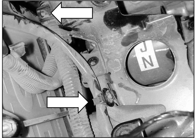
j. Unclip the wiring harness from the air box bracket behind the battery.
