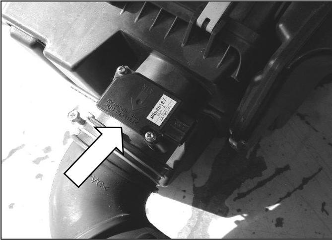
i. Remove the two bolts securing the MAF sensor to the air filter housing and remove the MAF sensor.
