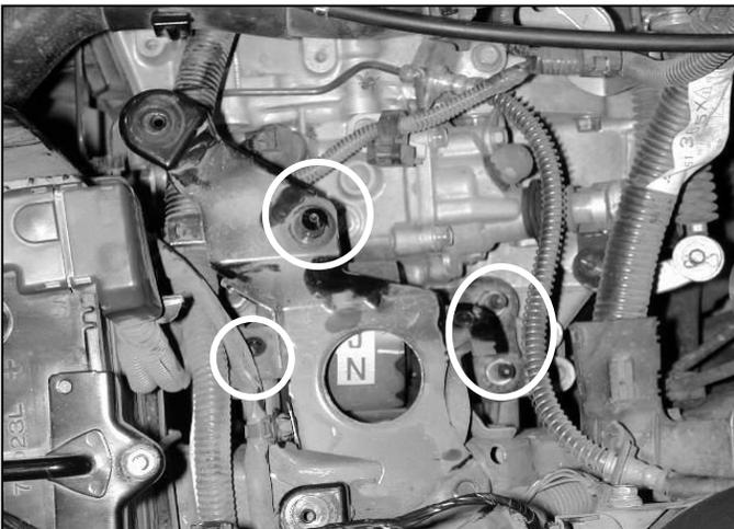
k. Remove the three bolts securing the air box bracket to the car. Remove the bracket.
