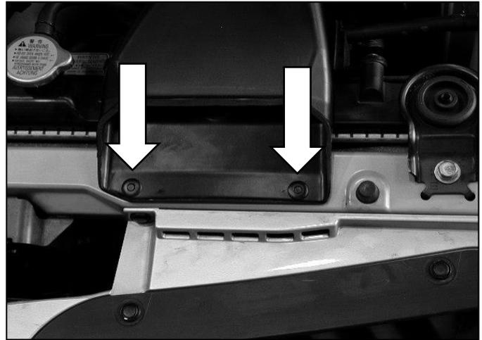
b. Remove plastic intake duct from the front of the engine by removing the plastic clips and pulling the duct straight forward. To remove the clips, use a pointed device and push in the middle of the clips.
