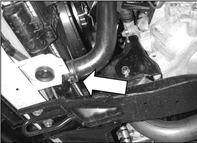
k. For best fitment, it may be necessary to loosen the spring clamp on the lower radiator hose and rotate the hose away from the lower intake pipe.
