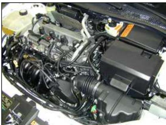
a. Factory airbox system installed.
