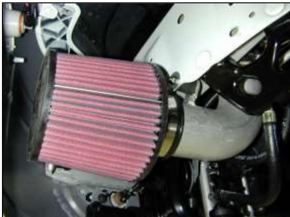
j. Secure the AEM® air filter onto the end of the lower intake pipe with the provided hose clamp.
