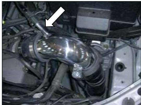
e. Install the upper intake pipe onto the throttle body. Attach the breather hose to the intake pipe's nipple.
