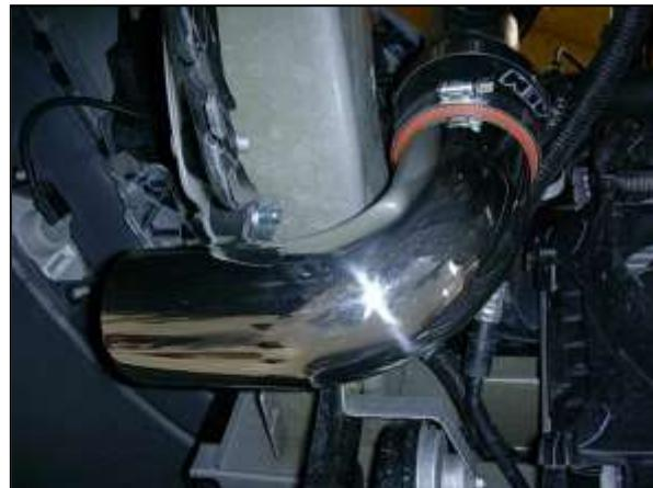
i. Install the lower intake pipe into the lower coupler of the MAF sensor housing. Align the intake pipe's bracket with the rubber mount secured to the frame rail.
