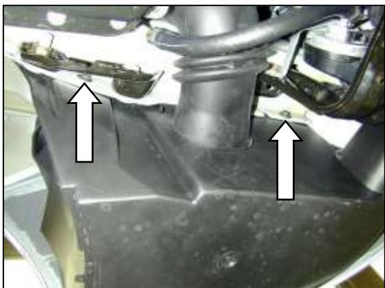
g. From underneath the vehicle, remove the two screws that secure the splash shield.
