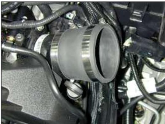
b. Install the rubber reducer with two hose clamps onto the throttle body.
