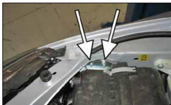
4. Remove the two nuts securing the factory airbox. Save these nuts for later use.
