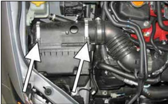
9. Unclip the airbox clips and remove the rear half of the factory airbox assembly.
