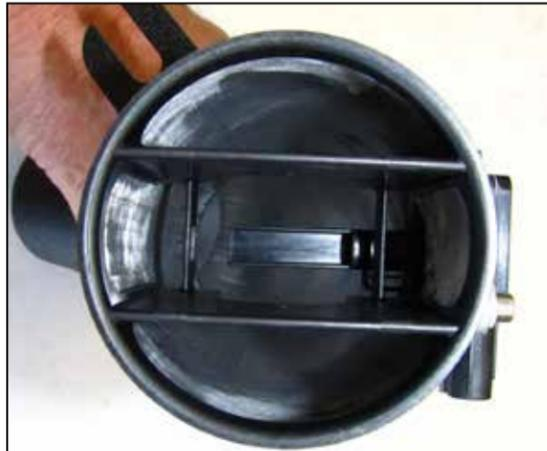
16. Apply four drops of the provided super glue around the lip of the maf insert and then insert the maf insert into the intake tube so that it aligns with the maf sensor as shown.
