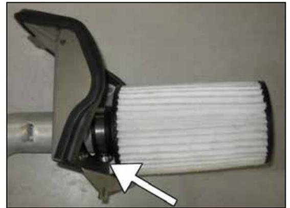
19. Orient the hose clamp as shown in the picture, and tighten.
