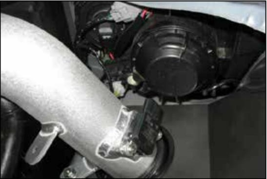
27. Replace the headlight access cover that was removed in step 2].
