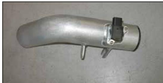
15. Install the MAF sensor in the AEM® intake pipe with supplied M4 screws.
