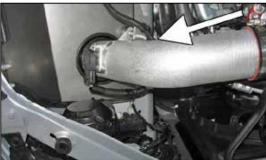
28. Route the MAF sensor wiring under the intake pipe, then secure the MAF sensor connector. Secure the MAF sensor wiring to the intake pipe's bracket with the tree-mount zip tie.
