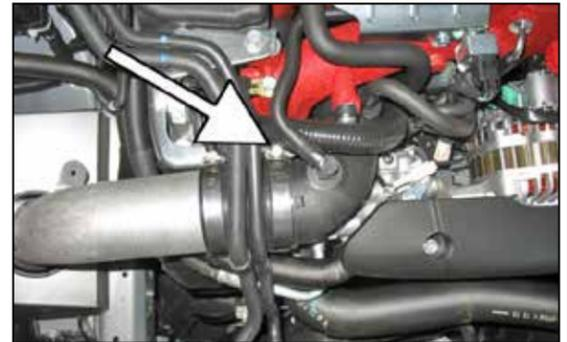
22. Slide the silicone coupler onto the compressor inlet pipe. Orient the hose clamps on the compressor inlet as shown and tighten securely.
