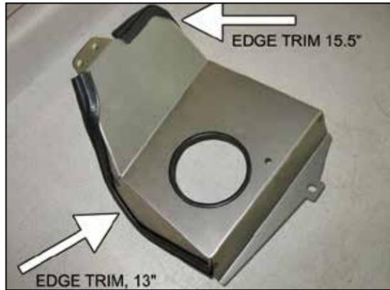
13. Install the rubber gasket trim on the heat shield as shown.
