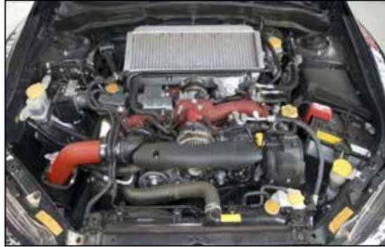
30. AEM® intake system installed
