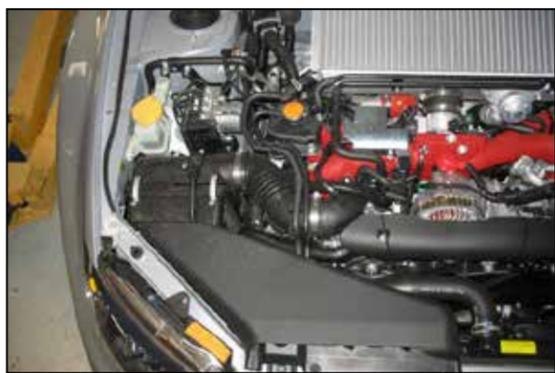
2. Remove the two plastic clips and factory fresh air inlet duct.
