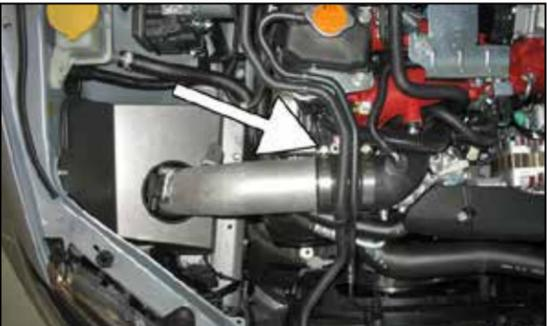
26. Hold the pipe in position and tighten the final hose clamp on the silicone coupler.
