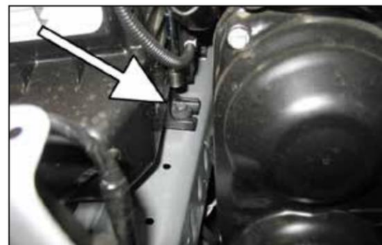
5. Remove the bolt securing the bottom of the factory airbox.
