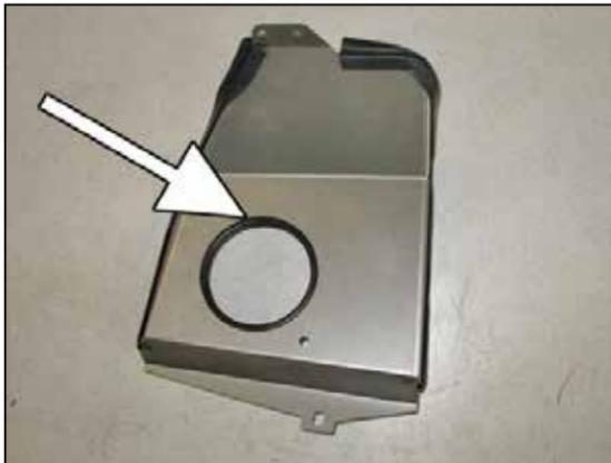
12. Install the rubber edge trim on the heat shield as shown.
