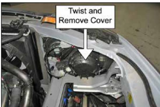
11. Remove the headlight access cover by twisting it counter clockwise. Save the cover for later use.
