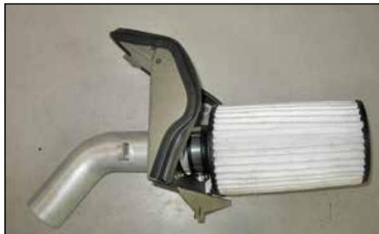
18. Slide the air filter and #48 hose clamp onto the end of the pipe until the pipe hits the intake pipe stop.
