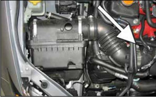
8. Loosen the hose clamp securing the factory airbox inlet to the compressor inlet tube.
