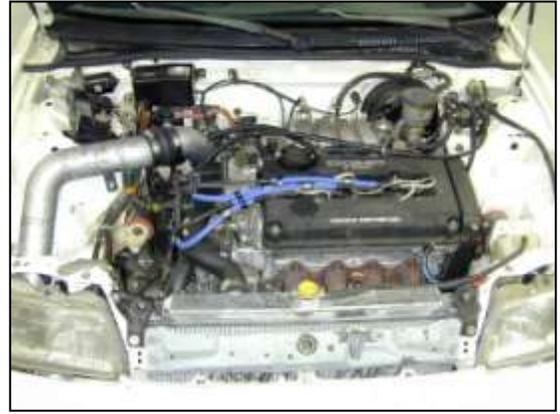
AEM® intake system installed
