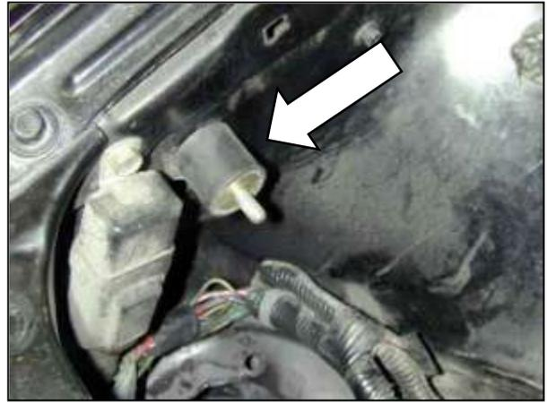
e. Insert the rubber mount in the location specified and tighten.
