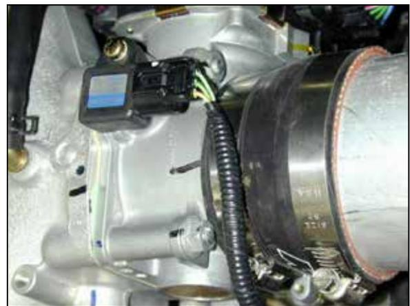
g. Install the silicone coupler attached to the AEM® intake pipe over the throttle body.
