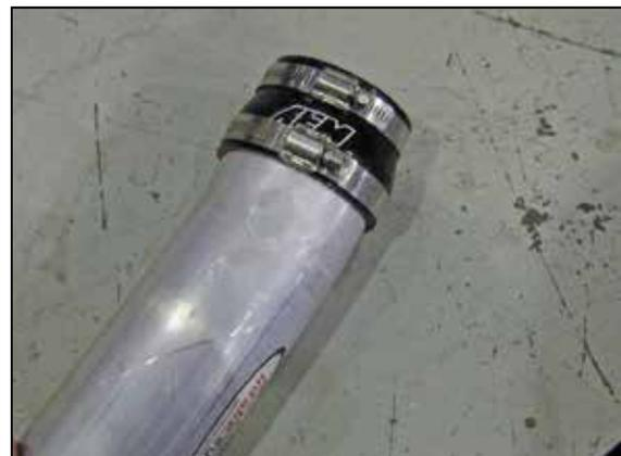
c. Check to see that the inside of the AEM® inlet pipe and air filter are clean and free from any foreign objects and/or obstructions. Install the 3"-3.25" silicone reducer over the throttle body end of the intake pipe using the 3" hose clamps.
