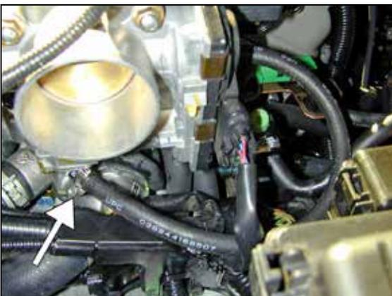
b. Install the provided 5/16" hose where the factory coolant line was removed. Use the supplied 3/4" hose clamps to secure the hose.
