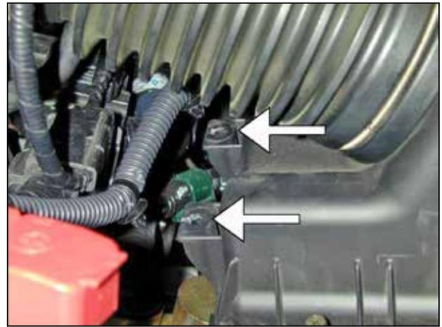
f. Remove the plastic clips holding the wiring harness to the throttle body side of the air filter housing.
