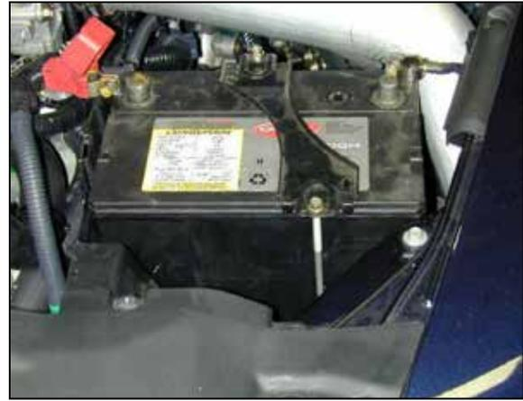
k. Reinstall the plastic battery under-tray, the battery, and the battery tie down bracket. Do not install the plastic battery cover. Check for proper clearance between the battery and the intake pipe. Use the supplied zip-ties to make sure no wires are in contact with the intake system.
