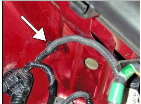
r. Release the wire loom from the hole in the fender.
