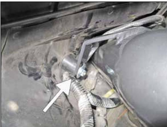
h. Guide the bracket on the intake pipe over the stud on the rubber mount. Once aligned, install the supplied washer and nylok nut onto the stud.
