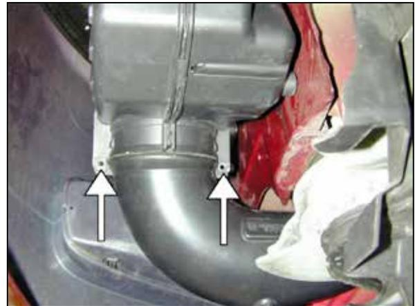
n. Removal of the stock intake resonator requires drilling. Start by drilling the two aluminum rivets shown.
