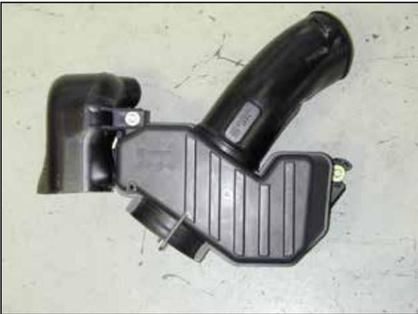
q. Remove the two bolts securing the resonator box to the frame. Remove the resonator box.
