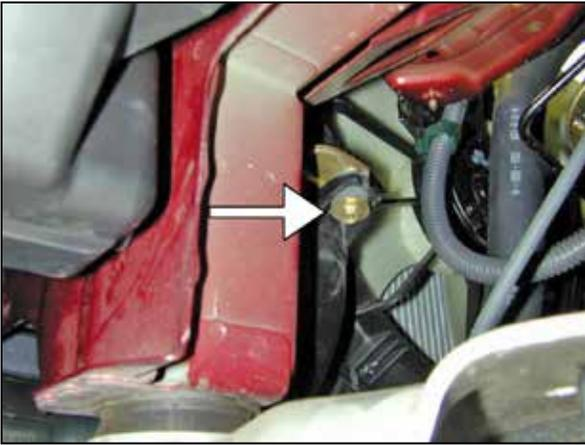
o. Remove the bolt securing the inlet tube to the frame. This can be reached through the wheel well.
