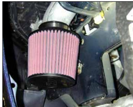
i. Install the AEM® air filter onto the end of the intake tube. Push the air filter over the intake pipe until the stop in the air filter is reached. Then install one hose clamp and secure the air filter onto the intake pipe. Once fitment is checked, tighten the hose clamp.
