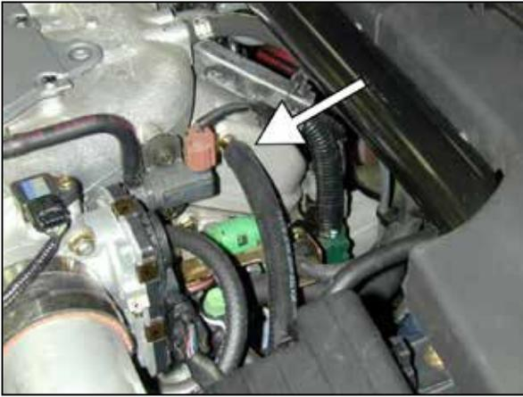
j. Install the supplied ½" breather hose between the intake pipe and the valve cover. Secure with provided 1" hose clamps.
