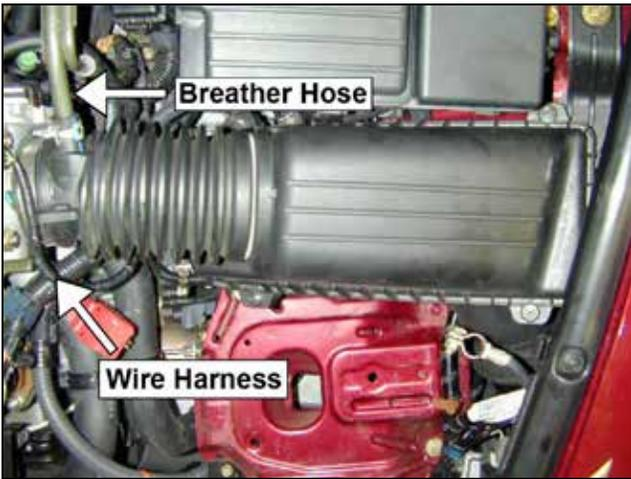
e. Loosen the hose clamp on the throttle body and unhook the wiring harness. Remove the stock breather hose from the inlet tube.
