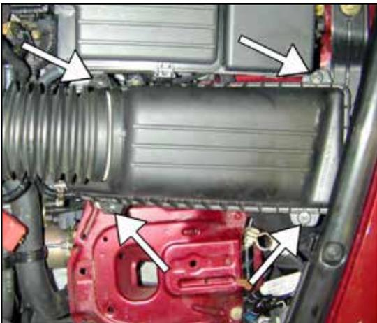
g. Pull the inlet tube off the throttle body. Remove the four screws holding the top of the air filter housing to the lower air filter housing.
