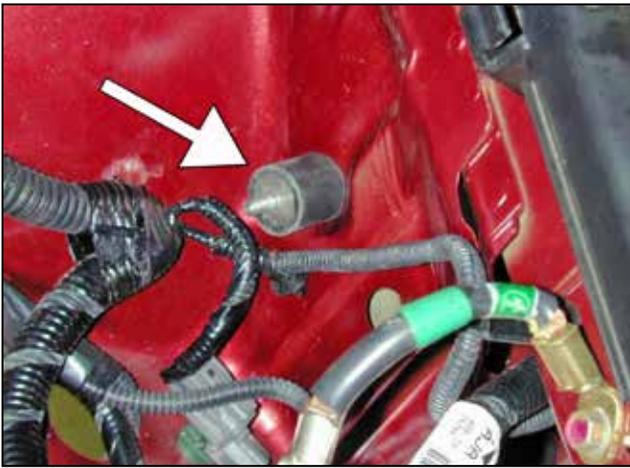
d. Install the rubber mount where the factory wire loom was removed.
