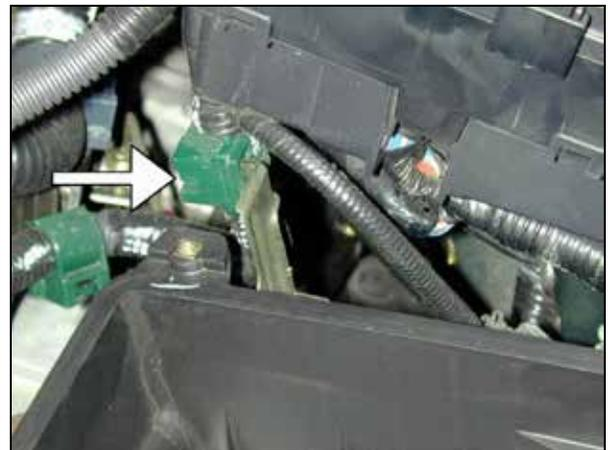
h. Remove wire clamp from the lower air box bracket.
