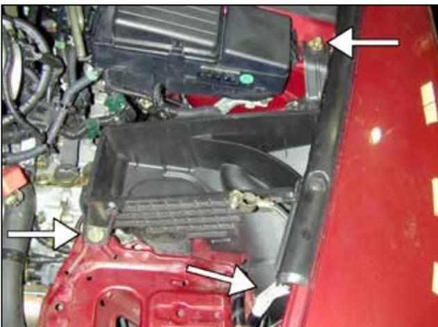
i. Remove the two bolts securing the lower air filter housing and remove housing. Pull up and remove the rubber sleeve connecting the air filter housing to the resonator below.
