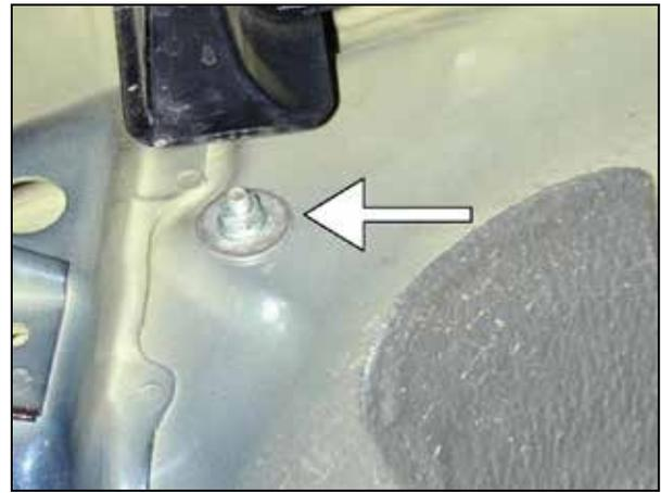
e. Secure the rubber mount using the supplied washer and nylok nut.
