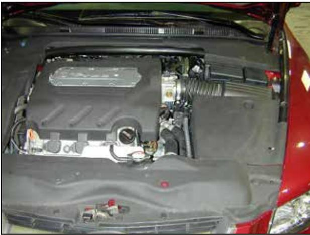
a. Factory air box system installed.
